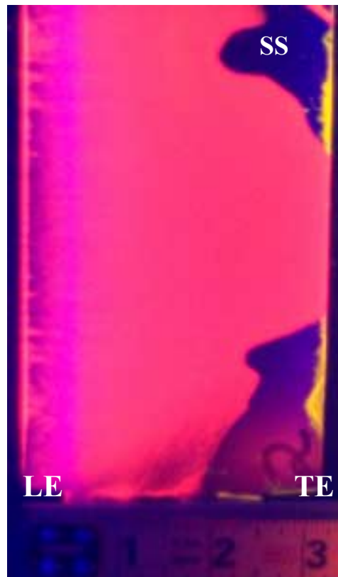
Figure 3. 4 Oil Visualization, I=44.4^\circ , M1\sim 0.65
