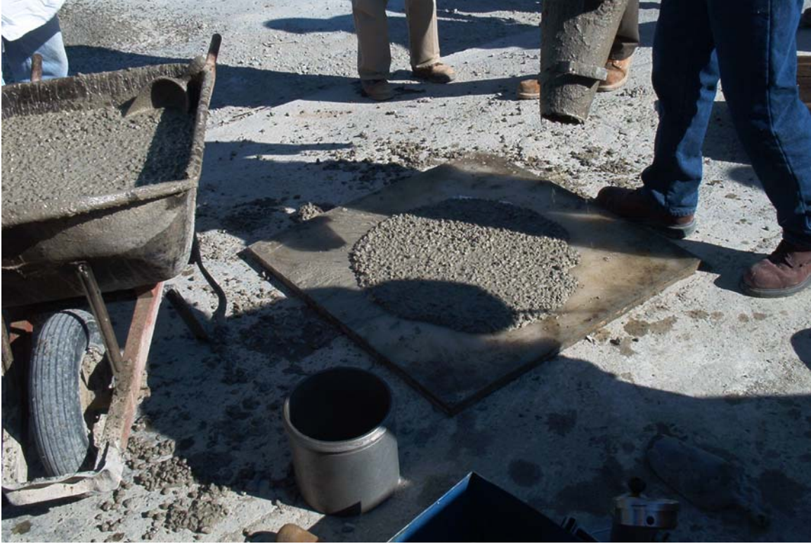
Figure 4-7. Slump test on batch of LWSCC concrete
