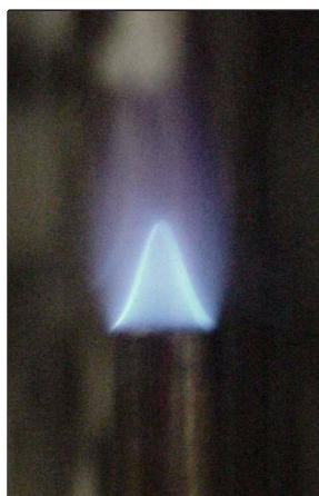
Figure 7.2: Photograph of stoichiometric Bunsen type flame
