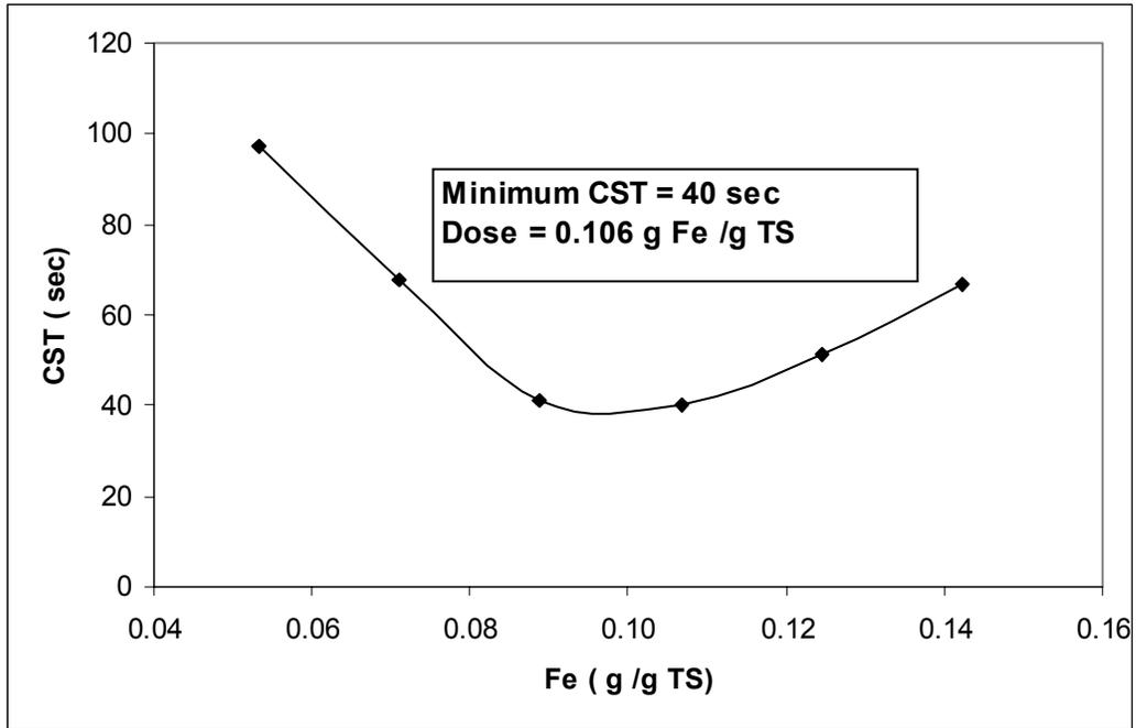
Figure 1: Dewatering using Ferric Chloride (Sludge from Cranberry, PA)
