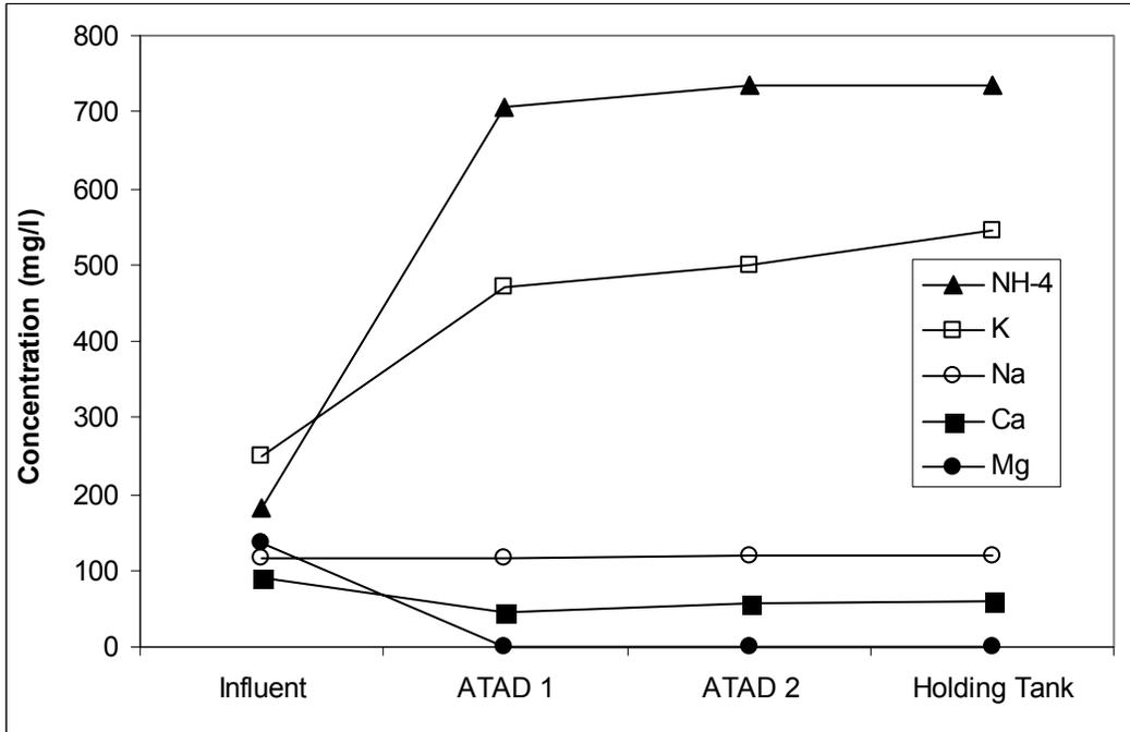
Figure 4: Changes in Cation Concentration in Solution Across the ATAD system (Titusville)
