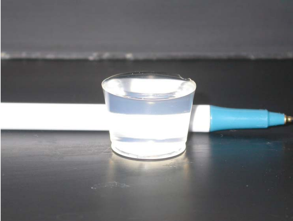
Figure 3.2.1: Sandia Xerogel after several months of ambient temperature and pressure drying
