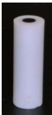
Figure 3-2. Glassy carbon electrode used for electrochemical experiments.
