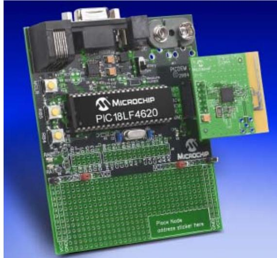
**Figure 2-4.** *PICDEM Z ZigBee Demonstration Board from Mirochip [16]*
