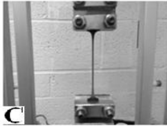
Figure 38: An example of (A) Dog-bone specimens. (B) Set the specimen for tensile test. (C) Tensile test.
