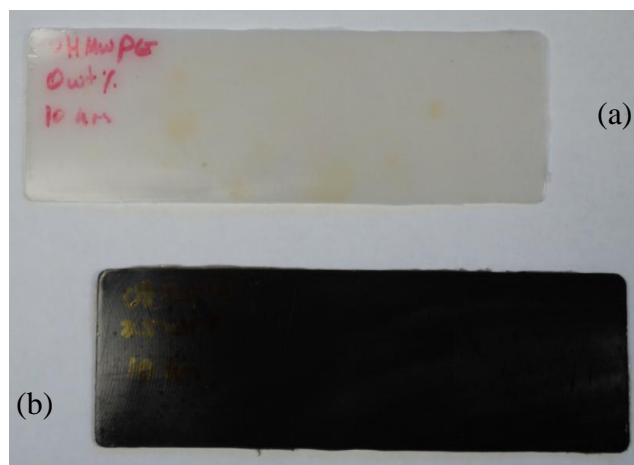
Figure 35: An example shows polymer sheets of (a) UHMWPE milled for 10h. (b) UHMWPE-2.5wt. % \text{Al}_2\text{O}_3 milled for 10h.
