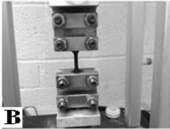
Figure 38: An example of (A) Dog-bone specimens. (B) Set the specimen for tensile test. (C) Tensile test.
