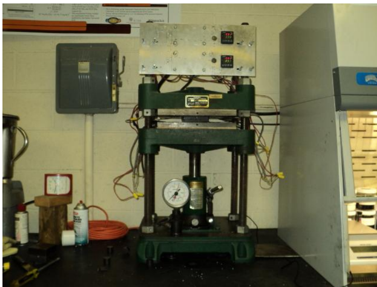
Figure 34: Carver press used for pressing polymer sheets. Professor Donald G. Baird's lab, Chem E VT, Blacksburg.
