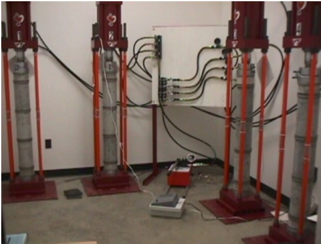
FIGURE 2C. CREEP ROOM: FOUR COMPRESSION FRAMES WITH THREE SPECIMENS PER FRAME.
