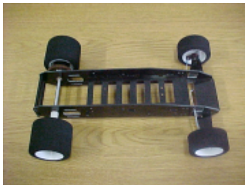
Figure C.2: The chassis on which the everything is build
