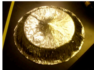
Figure 4-1-3b Perforated LiteLid® wrapped with aluminum foil (Photo by author, 2008)
