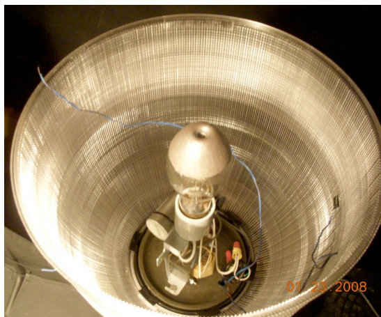
Figure 4-1-4a Reflective Paint on the tip of the 100W HPS lamp (Photo by author, 2008)
