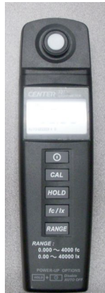
Figure 3-2-2a Center 337 Mini Light Meter - New Meter (Photo by author, 2008)
