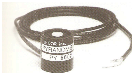
Figure 3-1-2a LI-COR Radiation Sensor Image (LI-COR Radiation Sensors Instruction Manual, 2009)
