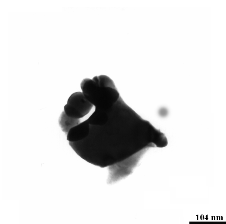
Figure 4.3 An Aggregate of Several Crystallites in a Sample Annealed at 1000 °C for 4 hrs Sample I.D.: w = 7.5 , [Y^{3+}] = 1.0 \text{ M} , [\text{NH}_3] = 5 \text{ M} , [\text{AOT}] = 0.1 \text{ M}
