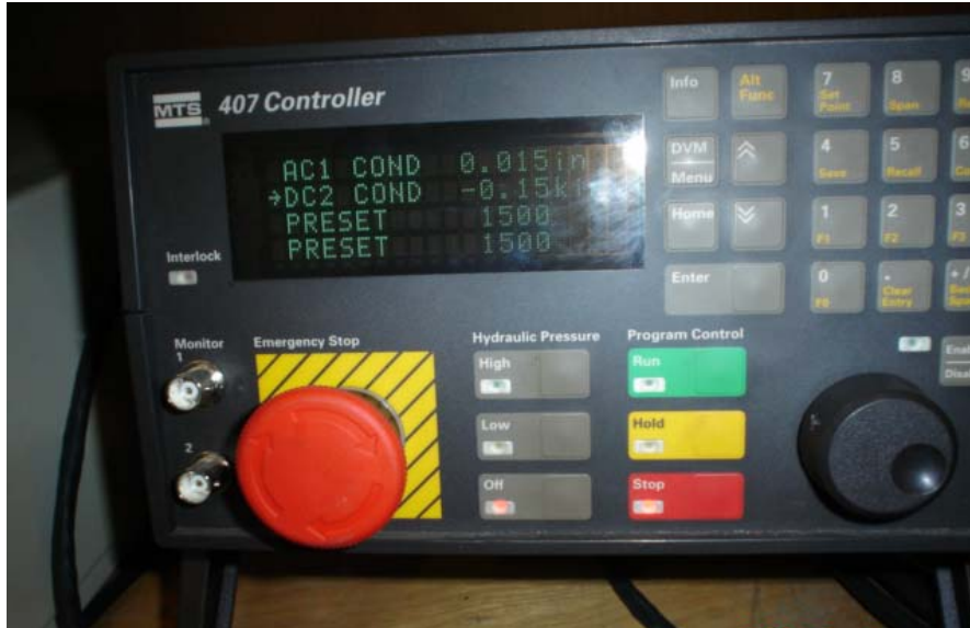
Figure 3.8: MTS 407 Controller for Universal SATEC Machine
