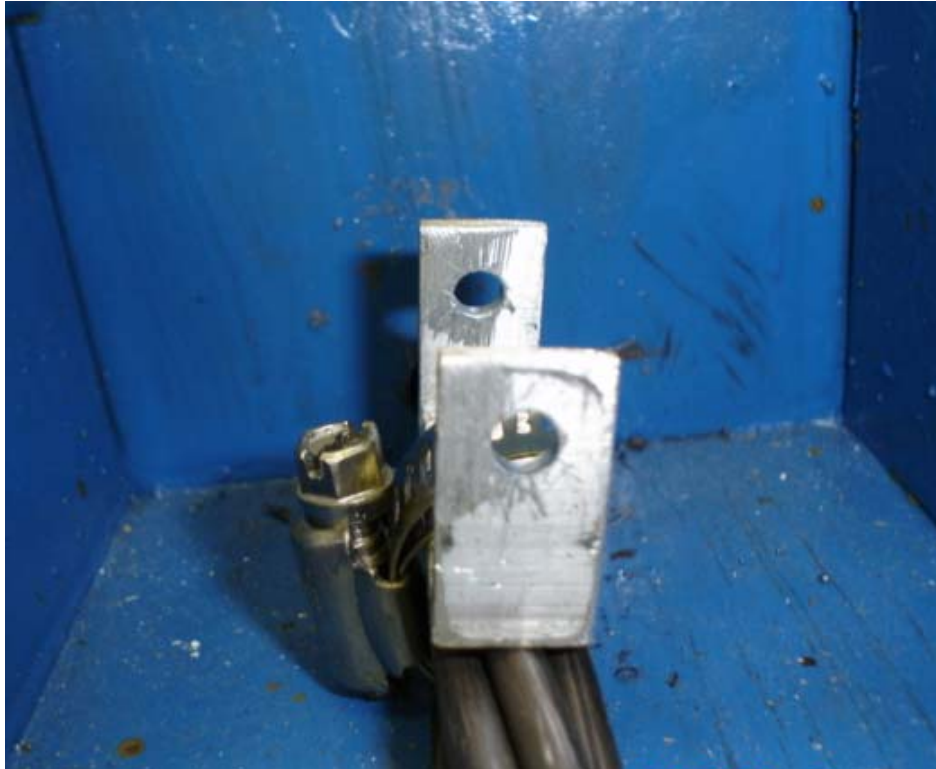
Figure 3.19: Aluminum Angle for Depth Micrometer
