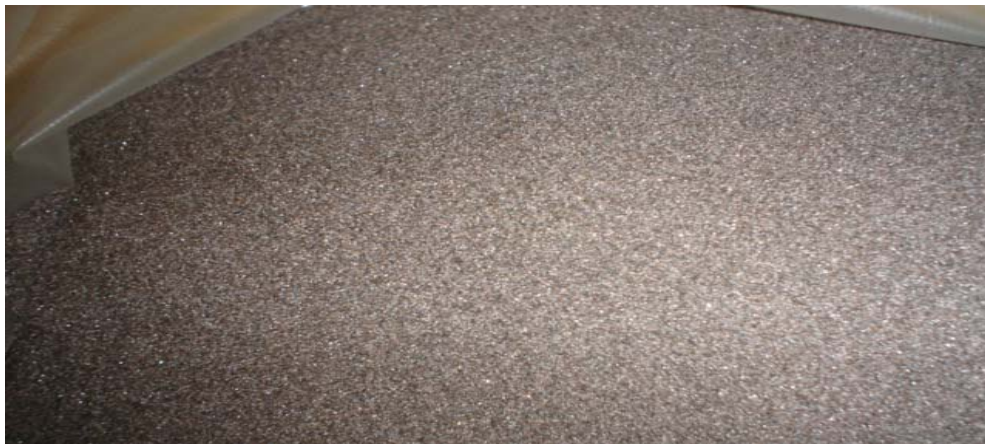
Figure 3.5: 80 Grit Aluminum Oxide
