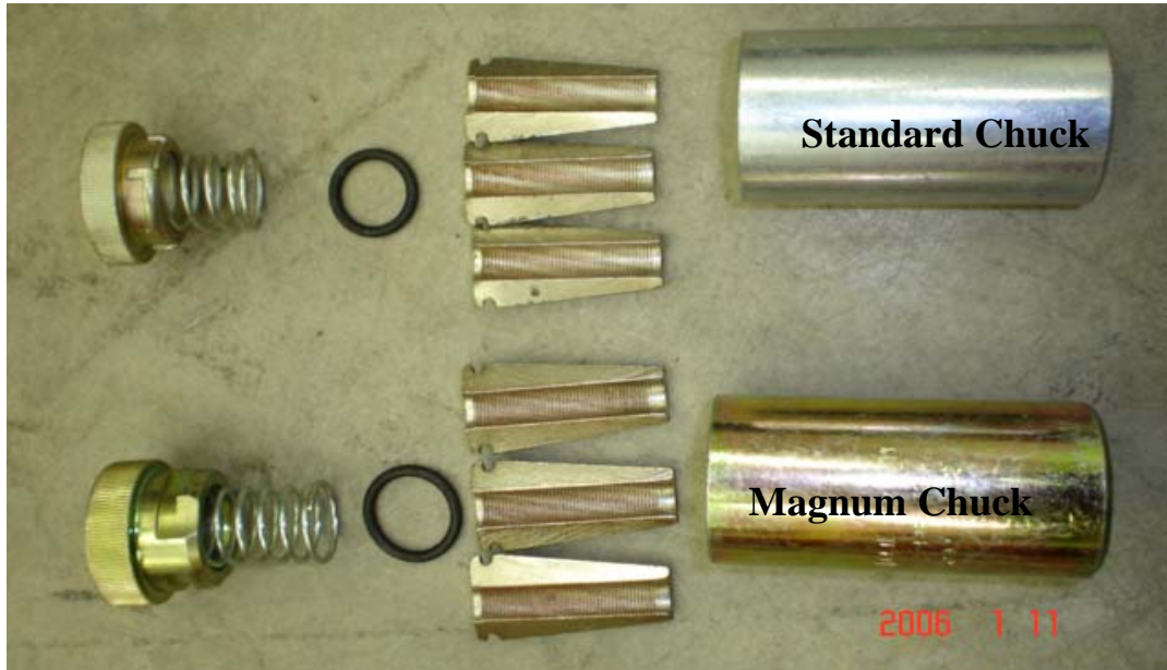
Figure 3.15: Comparison of Standard and Magnum Chucks
