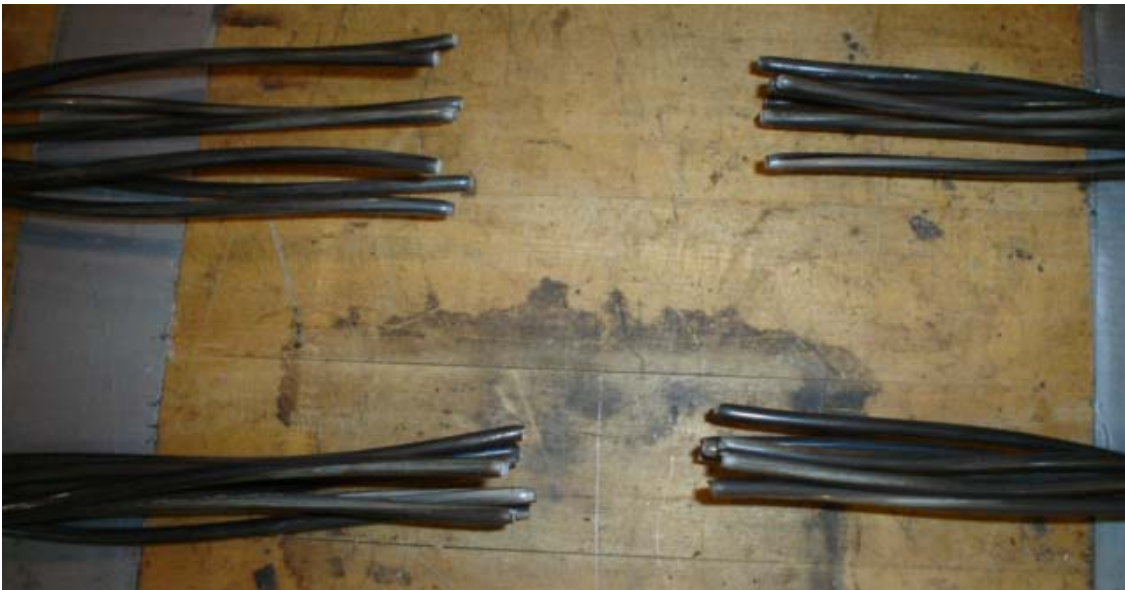
Figure 4.12: Clear Breaks in Center of Strand
