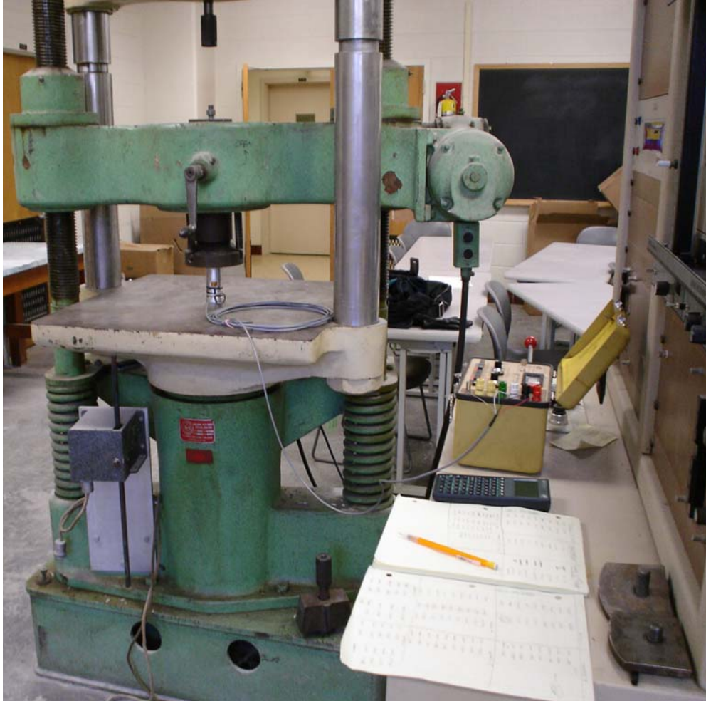
Figure 3.17: Load Cell Calibration
