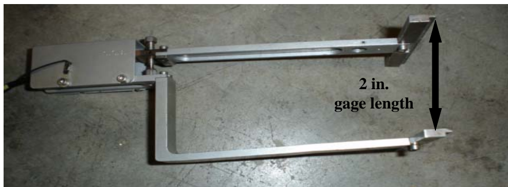
Figure 3.7: SE2-50 Extensometer with 2 in. Gage Length
