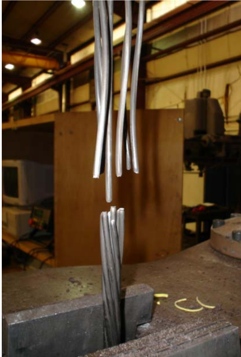
Figure 4.13: Clear Break in Test Machine
