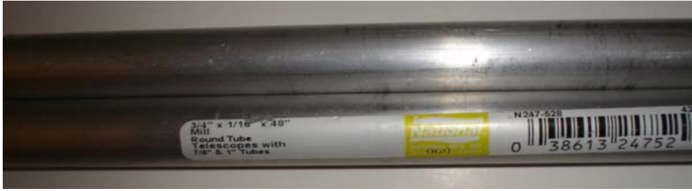
Figure 3.4: Aluminum Round Tubing 3/4 in. x 1/16 in. x 8 in.
