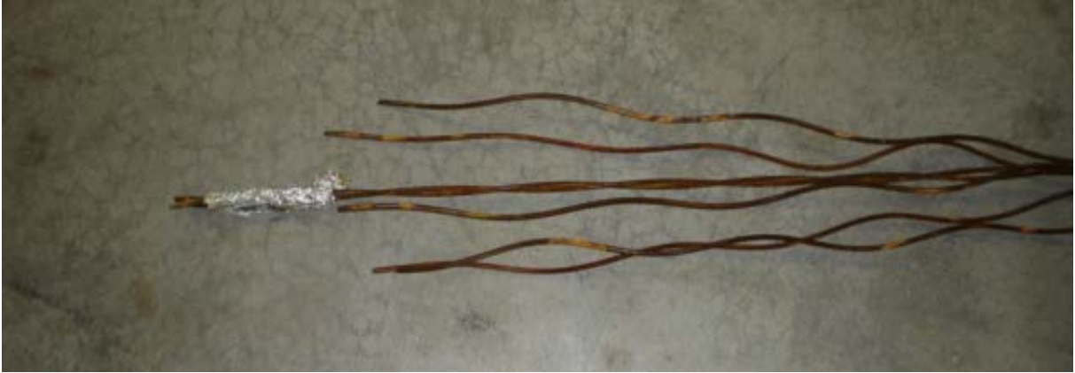
Figure 4.11: Break at Grips using Aluminum Foil
