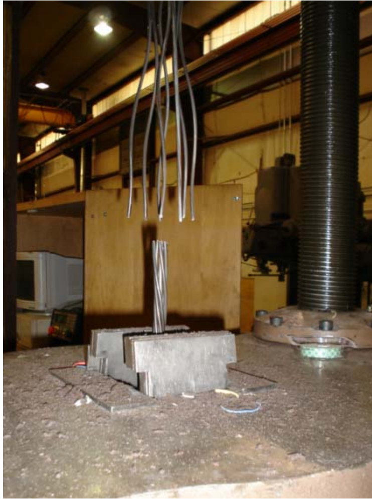
Figure 3.10: Fractured Strand in SATEC Machine
