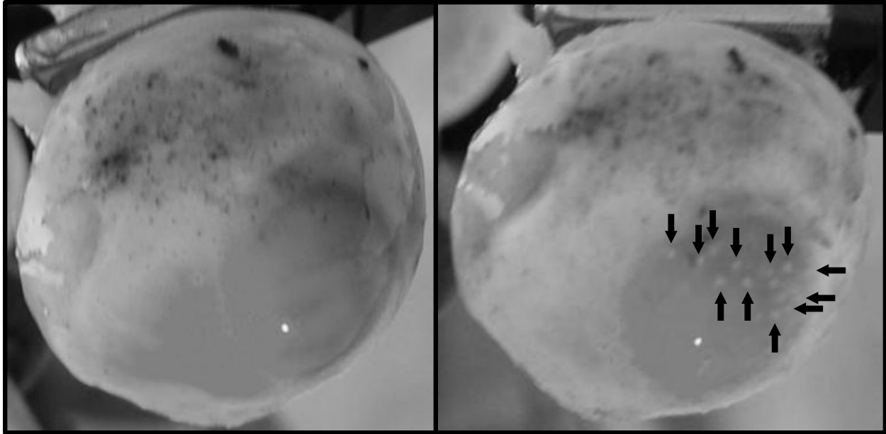
Figure 12. (Left) Photograph before 5 cm standoff distance test. (Right) Post-test photograph with arrows indicating corneal abrasions. Fluorescein dye used to better visualize corneal abrasions under a blue light. Bright white dot is a reflection of light.
