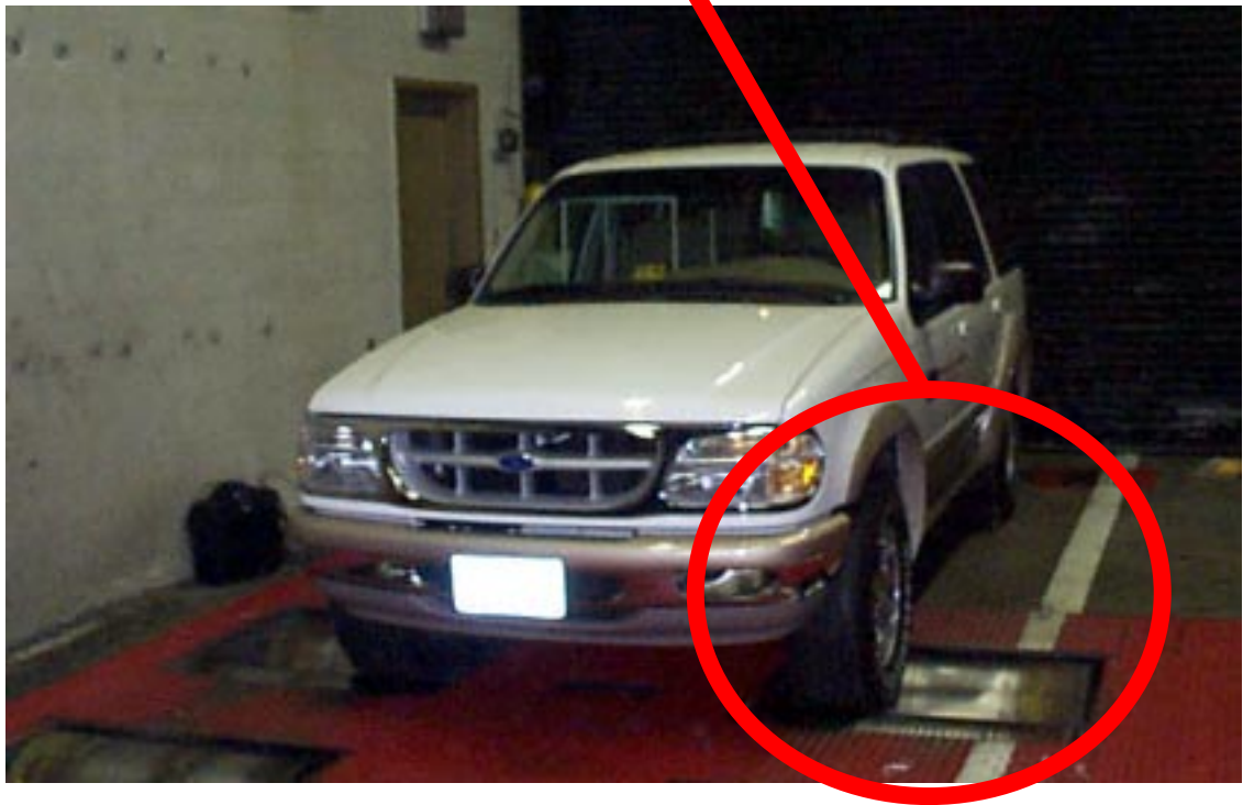
Figure 5.32 Test rig for the Volvo dynamometer experiment
