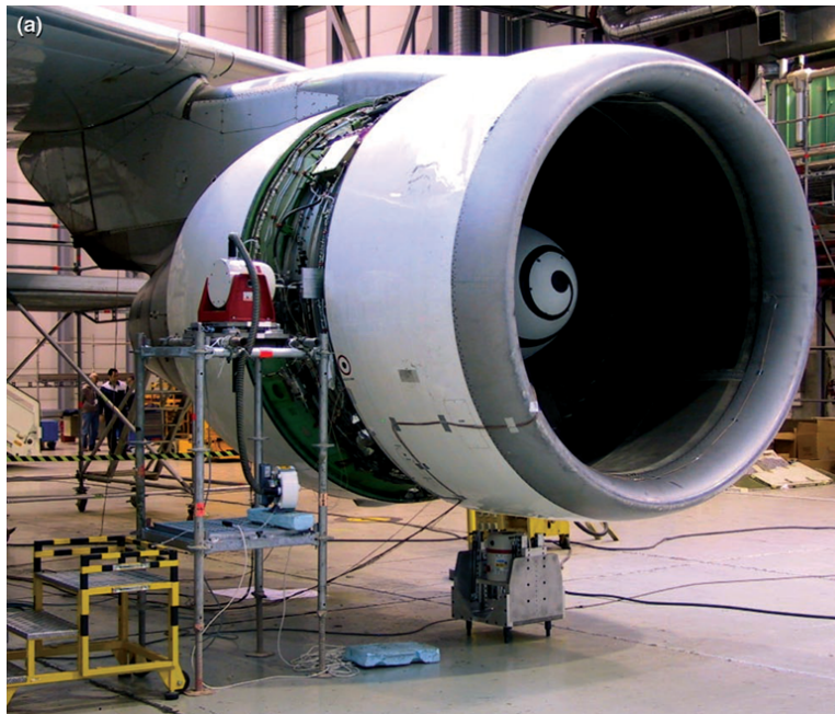
Figure 5.1: Shaker excitation of aircraft engine[6].
