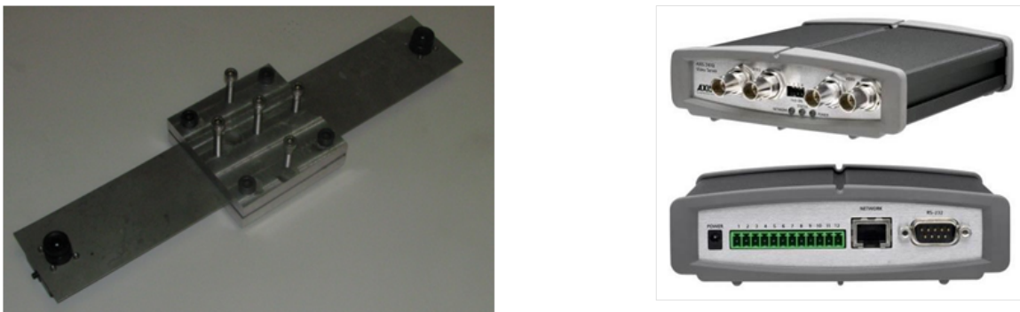
Figure 4.1: Stereo System with two Watec 660D cameras and Axis 241Q Video Server.
