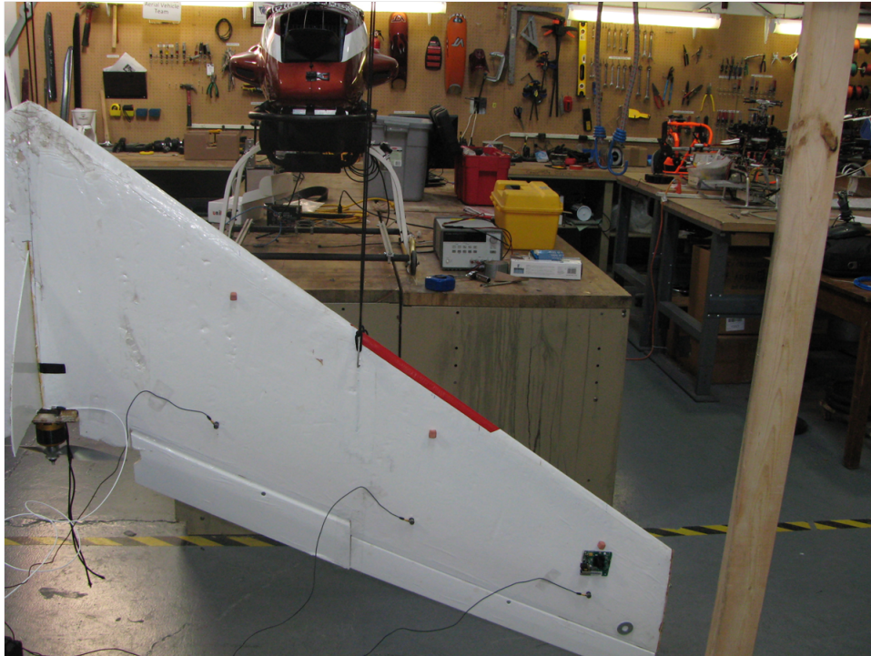
Figure 5.5: Close-up showing accelerometer and dummy mass placement.
