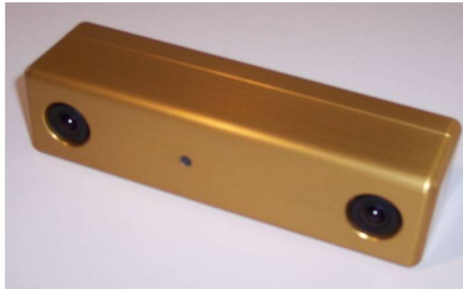
Figure 2.3: Example of stereovision system [3].
