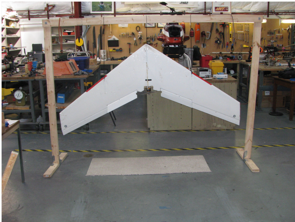
Figure 5.3: Experimental flying wing suspended from wooden frame with bungee cords.
