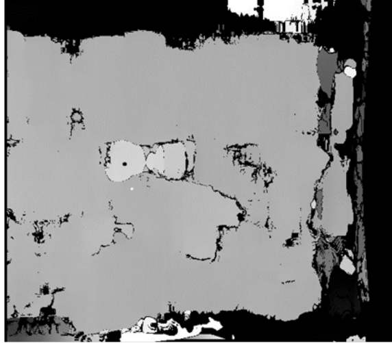
Figure 4.8: Disparity map from correlation without vibration and correction angle.
