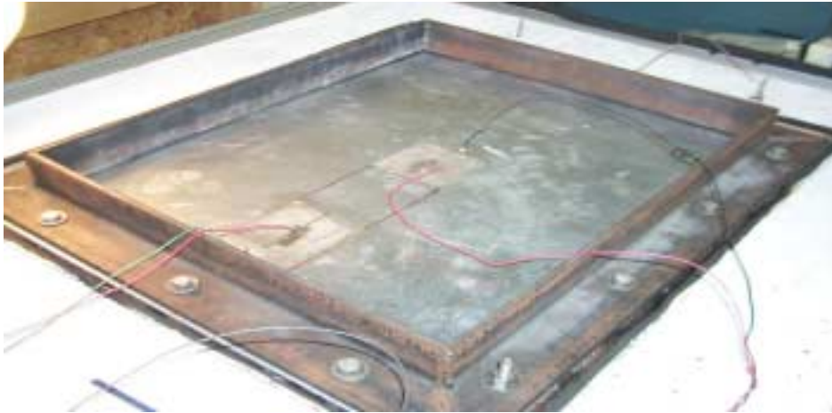
Figure 4.11. Smart Test Plate for Active PZT Tests
