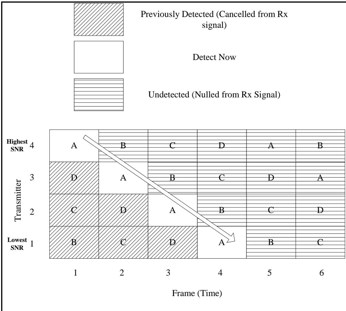
**Figure 2-6: The relationship between data streams and transmitter antennas. The transmitter numbering constitutes the spatial dimension of the space-time system.**
