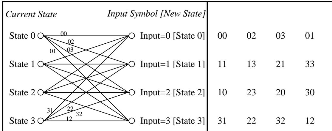
**Figure 2-4: Space-time trellis code (left) and an output table (right) for an  $n_T=2$ , 4-ary system with four states.**
