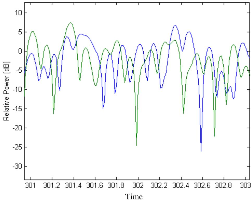
**Figure 2-1: The simulated envelopes of two uncorrelated Rayleigh fading signals**
