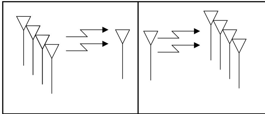
**Figure 2-2: Arrangement of antennas in diversity systems. Left: Transmit diversity, Right: Receive diversity.**
