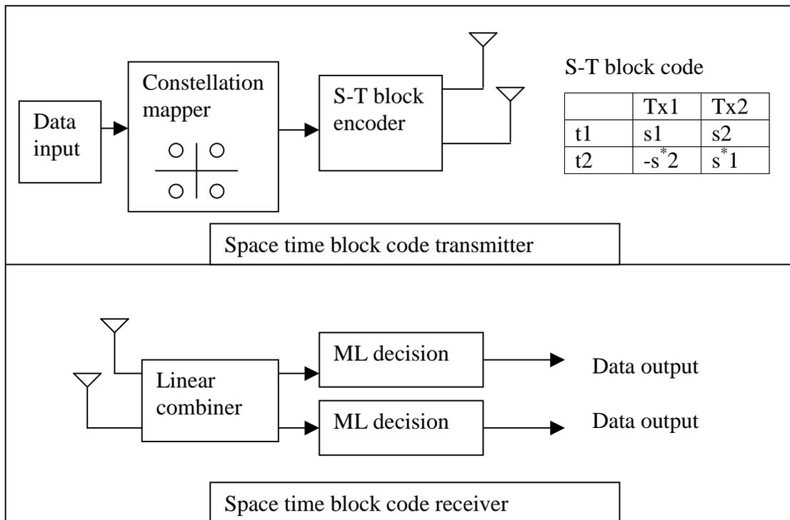
**Figure 2-3: Block diagram of a space-time block code transmitter and receiver**
