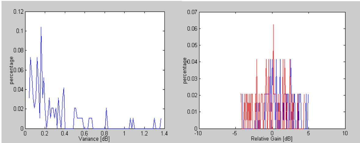
**Figure 5-2: Distribution of the mean and variance values of the received power for the daily calibrations. Each mean or variance value represents the statistics of gain over a ten second measurement for a single channel at a single measurement location.**
