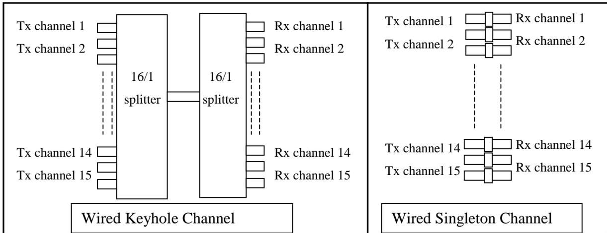
**Figure 5-3: Cable arrangements between the transmitters and receivers, producing the wired keyhole (left) and wired singleton (right) channels. All signals pass through a single cable to produce the keyhole channel, and all of the signal paths are independent in the singleton channel.**
