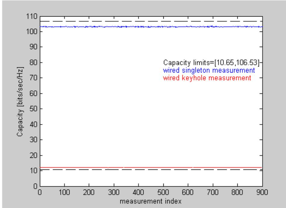
**Figure 5-4: Measured capacity values in the wired keyhole (red) and wired singleton (blue) channels. The theoretical upper and lower capacity values (black) were calculated from the identity matrix and the all-ones matrix, respectively.**
