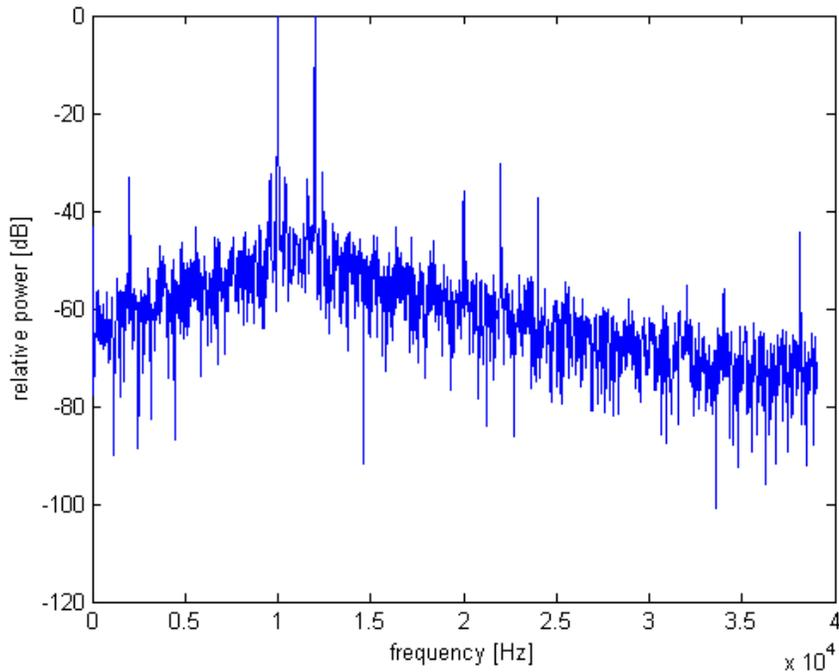
**Figure 5-1: Power spectrum calculated from the sampled data recorded by the receiver.**
