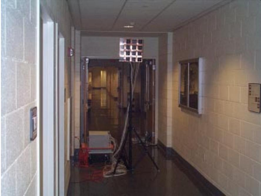
**Figure 6-5: Transmitter subsystem in the Hallway environment.**
