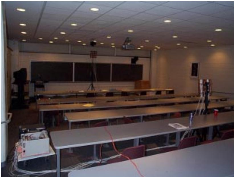
**Figure 6-12: Receiver subsystem and the transmitter array in the lecture hall environment. The transmitter subsystem is hidden behind the front row desk.**
