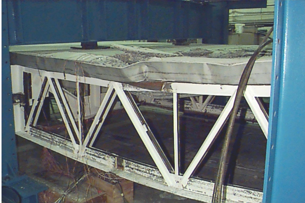
Figure 3.31 Buckling of EG Top Chord and Bottom Chord Yielding Between Third Points (FF-2)
