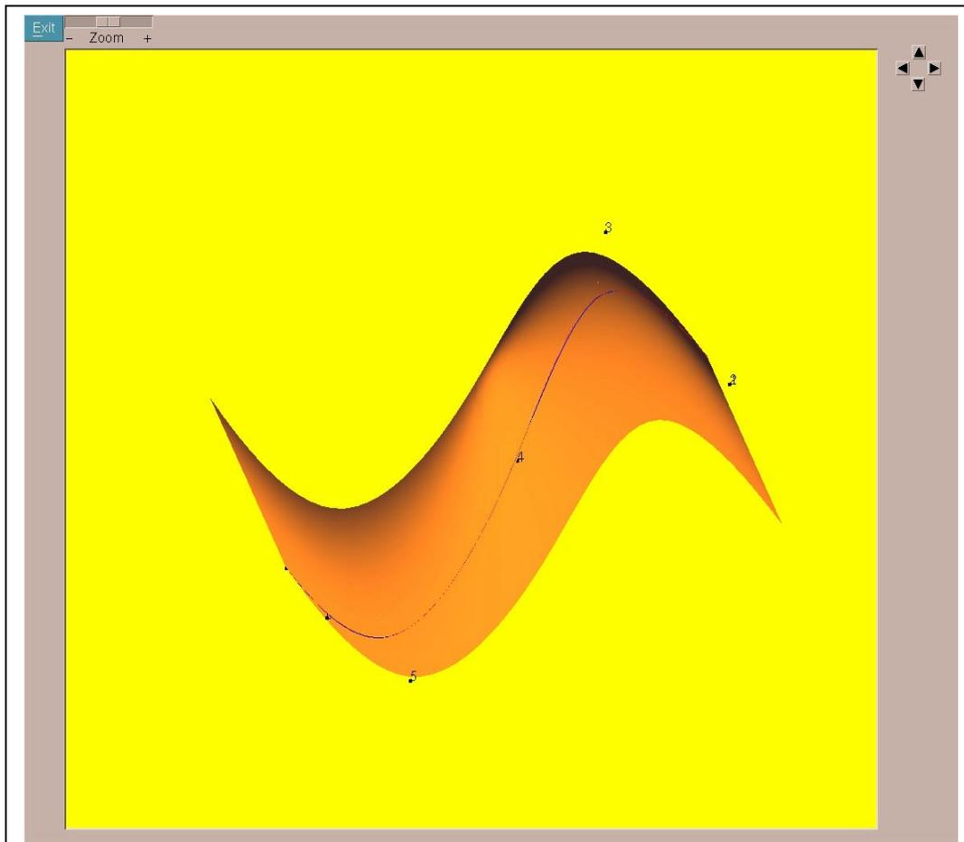
Figure 6.1: A screen shot of the interface developed using X/Motif. An OpenGL context is set to the window to enable OpenGL commands to take effect.
