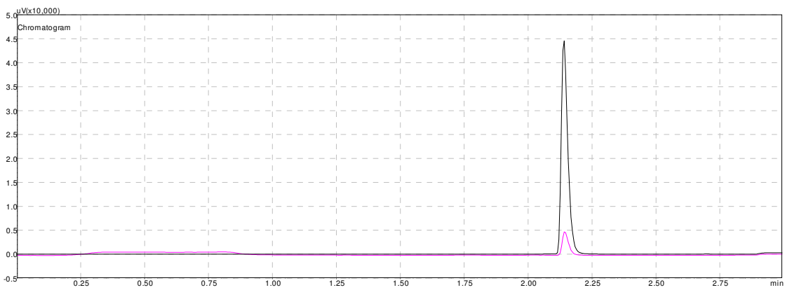
Figure B. 12: Comparison of Oxygen Peak (black line) with 10µL Pure Injection of CF 4 (pink line)
