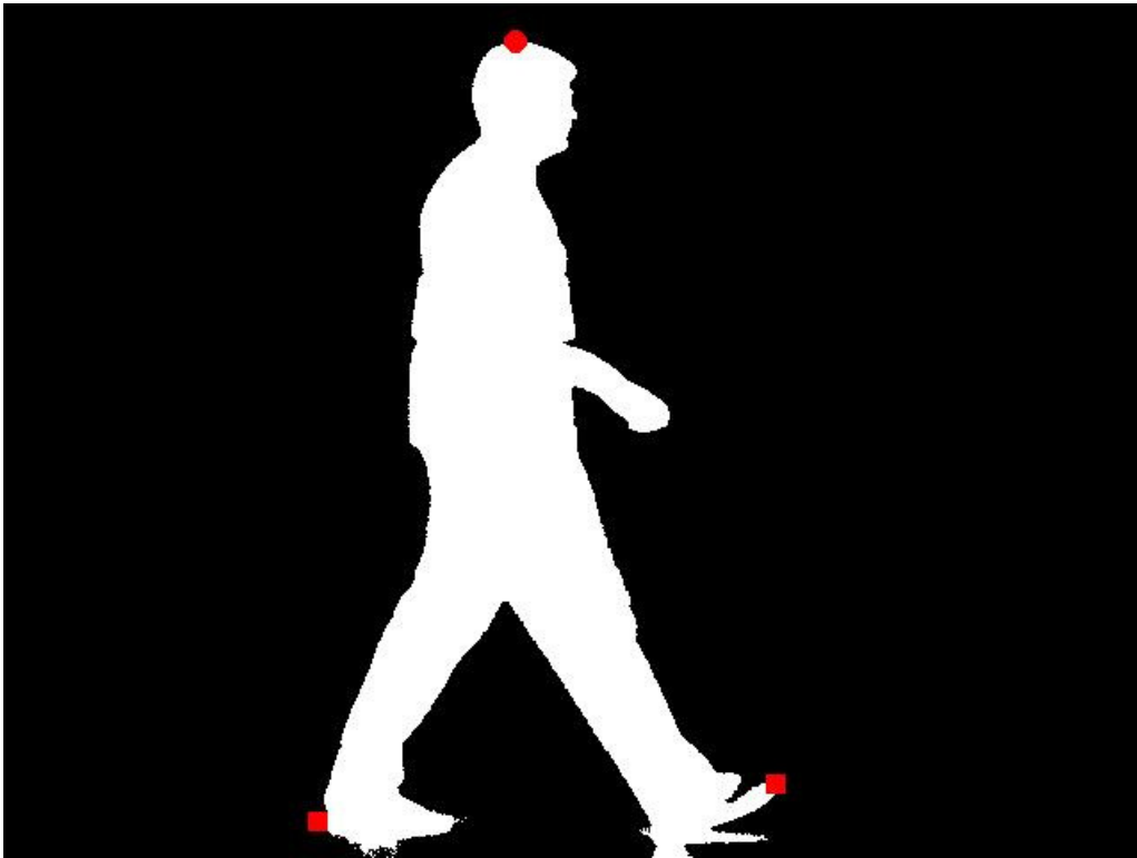
Figure 5.13: The point that is used for approximate height is shown as a red square and the two points used to calculate stride length are shown as red squares, both are superimposed on the binary silhouette which was used to calculate the values
