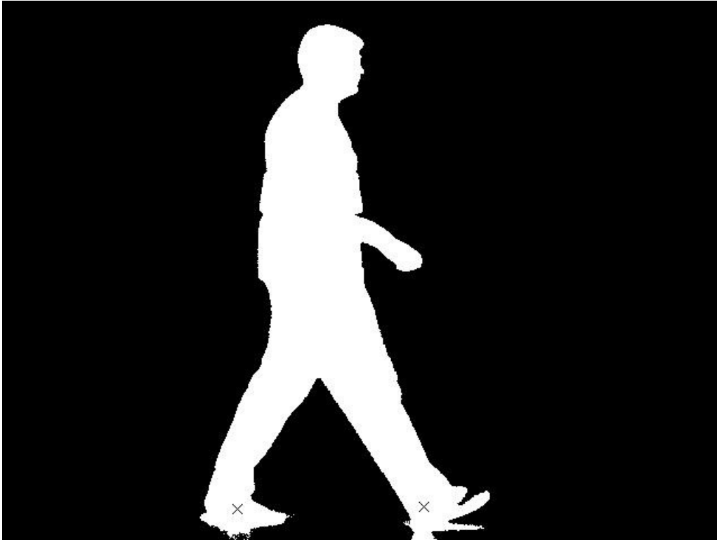
Figure 5.8: Foot centroids shown as an 'x' superimposed on a binary silhouette
