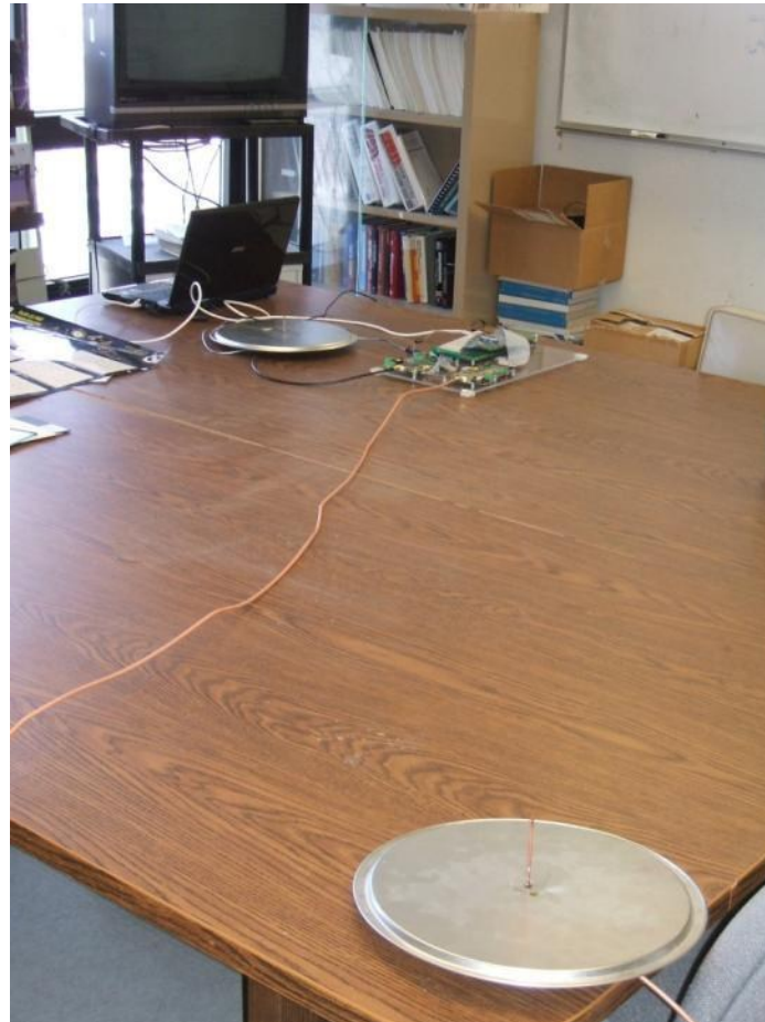
Figure 5.23: Test setup for line-of-sight test
