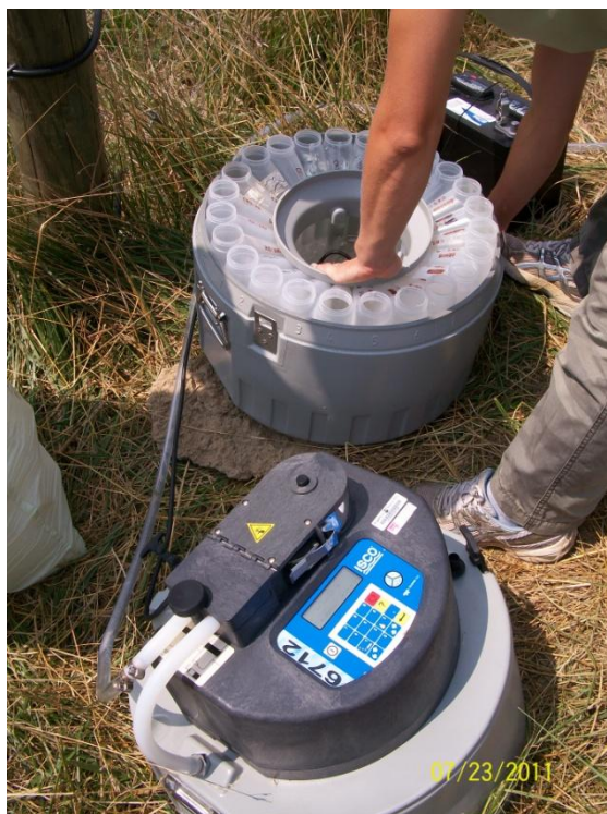
Figure 3.5: Automatic sampler (ISCO 6712) with 24 1-L bottles. (Source: Nancy Maschke)
