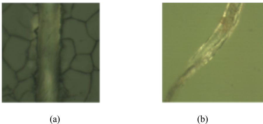
Figure 3 Optical microscopy pictures of fibers with (a) high hydrolyzed gliadin and (b) high myoglobin content. Fibers are 10 \mu\text{m} across.
