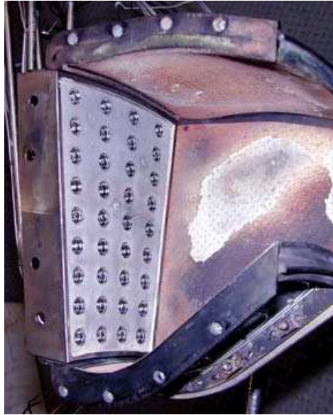
Figure 1.1: An LDI injector array in a sector combustor at NASA GRC.
