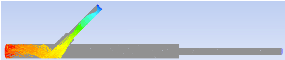
Figure 50. CFD Simulation of G 1 Particle Injection Path [44, 48]
