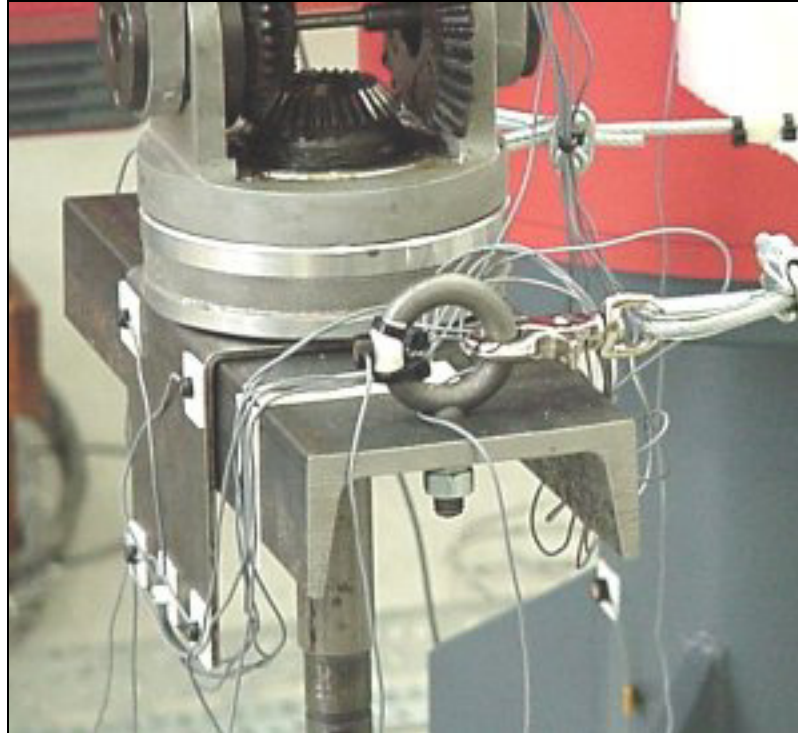
Figure 4.7 Regime Three Cable Sensor Mounting
