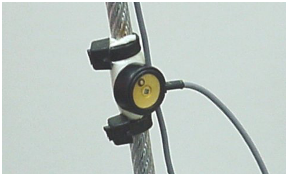
Figure 4.6 Cable Sensor Mounting Technique
