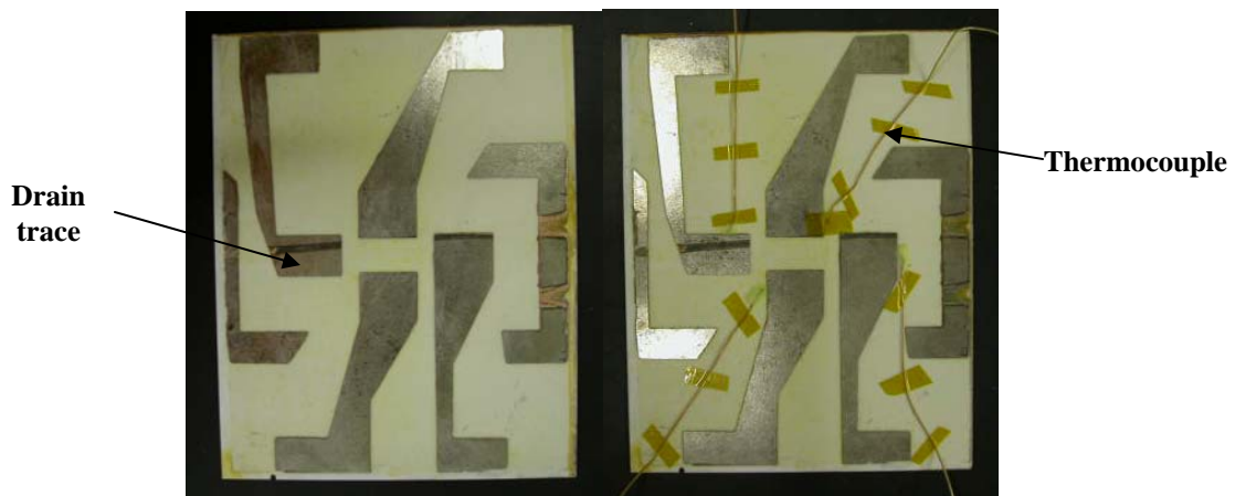
Figure 3.17 Drain pattern on DBC and DBC base with thermocouples
