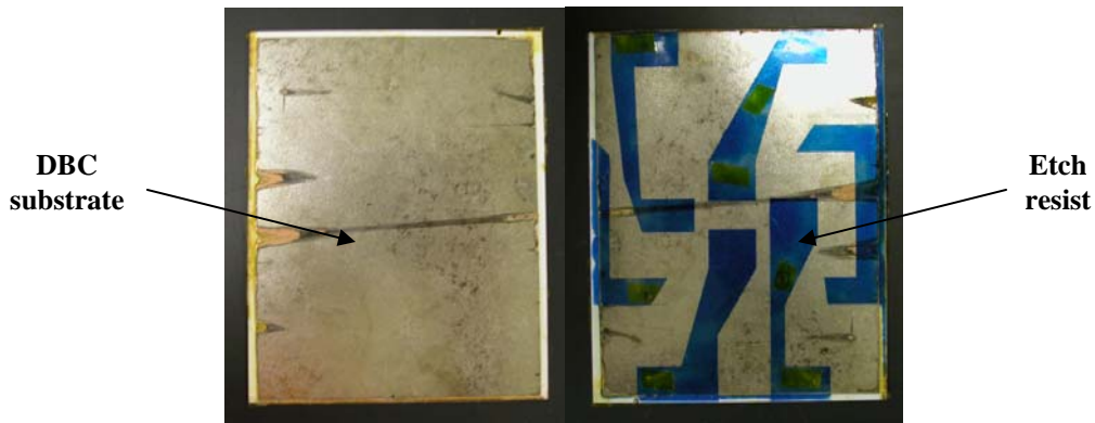
Figure 3.16 DBC and photo masked pattern on DBC
