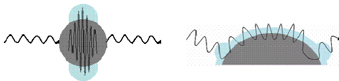
Figure 2.5: Incident light on nanostructured metal surfaces can generate localized (standing) plasmon resonances (left) as well as surface waves (right). Excitation of conduction electrons produces local electromagnetic fields near the metal surface.
