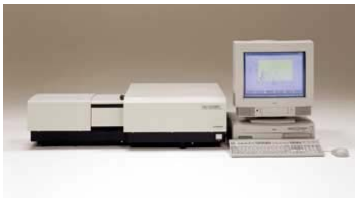
Figure 4.1: Shimadzu UV-3101PC UV-vis-NIR scanning spectrometer.
