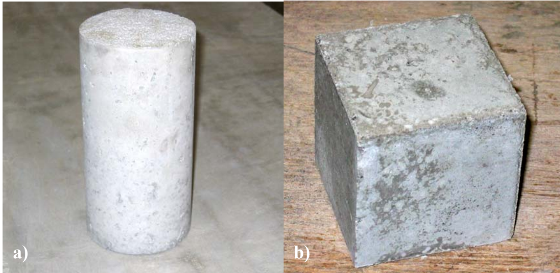
Figure 3.1: a) 4 in. x 8 in. Concrete Cylinder b) 2 in. mortar cube
