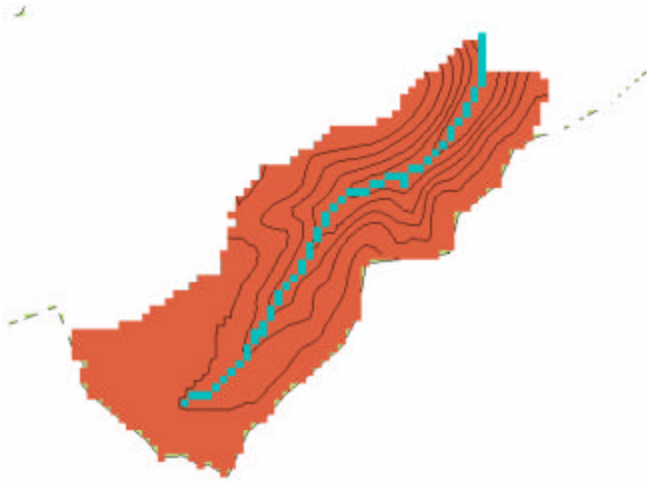
Figure 5.17: Contour Crenulation network in sub-watershed 5(12.5 ha) in the Surry 3 quad, with a minimum analysis unit of 10 ha.
