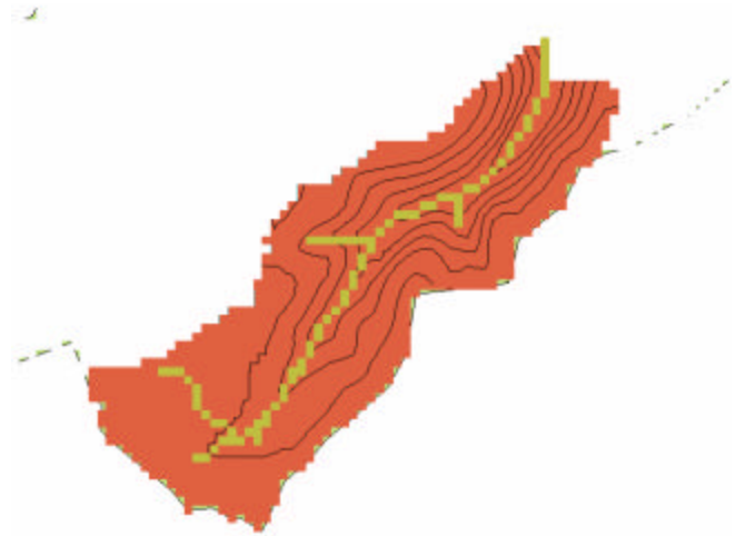
Figure 5.18: Terrain curvature network in sub-watershed 5 in the Surry 3 quad, with a minimum analysis unit of 10 ha. Percent error -3.6%.
