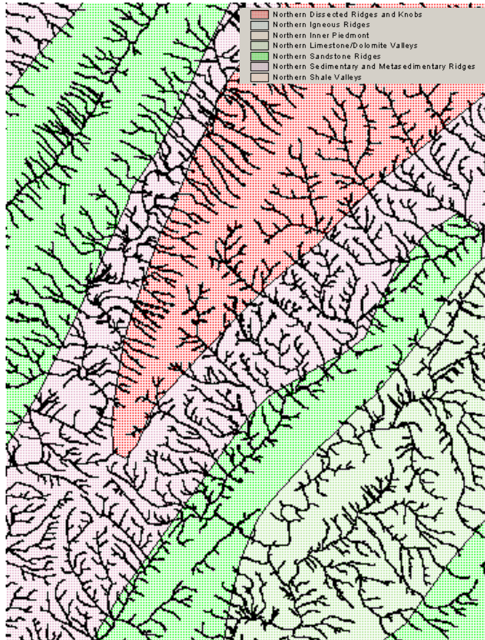
Figure 4.3: The networks predicted by the Ridge Accumulation method with eco-regions overlaid for the Craigville quad. Longest overland flow lengths are predicted in the Northern Sandstone Ridges (in green), which the shortest lengths are predicted in the Northern Shale Valleys (light tan, occupying the diagonal from the bottom left to the upper right of this figure).
