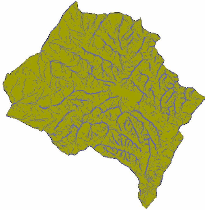
Figure 2.10: A ridge weight grid for the Briery Branch 2 sub-watershed. Cells in blue are cells whose flow accumulation value is zero (0) or “ridge “ cells, and are assigned a weight of one (1).
