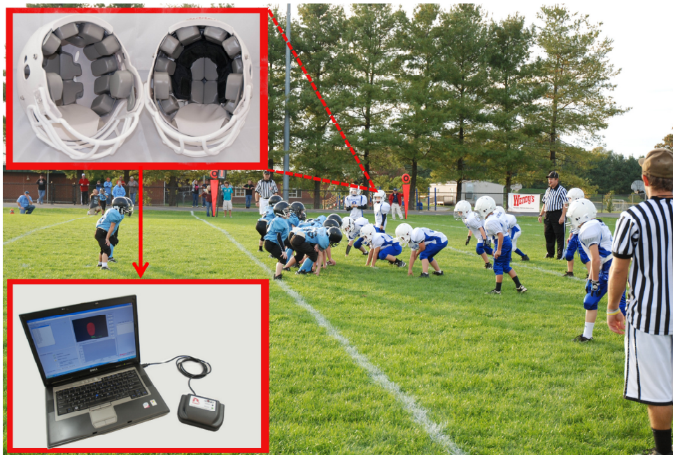
Figure 3. The helmets of youth football players were instrumented with the 6DOF head acceleration measurement device. Each time an instrumented player experienced a head impact, data were collected and then wirelessly transmitted to a computer on the sideline (Photo by author, 2012).
