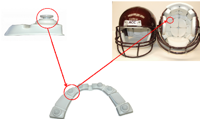
Figure 1. The 6 spring-mounted accelerometer sensor records resultant accelerations for every impact that a player experiences (Photo by Steven Rowson, 2010, Used with permission.)
