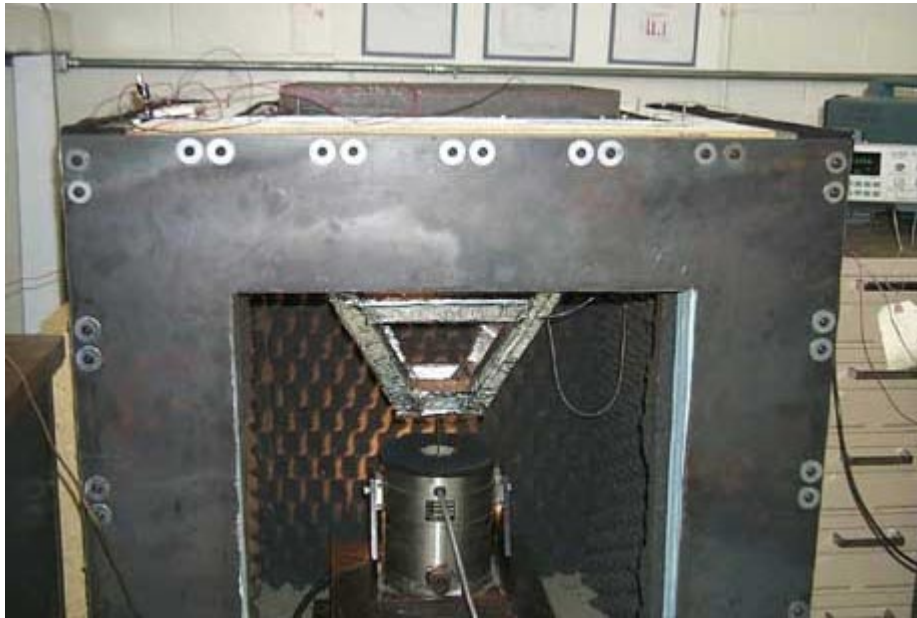
Figure 1.1. Vibration Test Stand with Electromagnetic Shaker and Excitation Frame.
