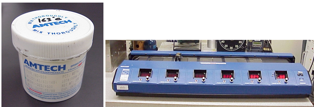
Figure 3.3. NC-559 paste and the reflow soldering system.
