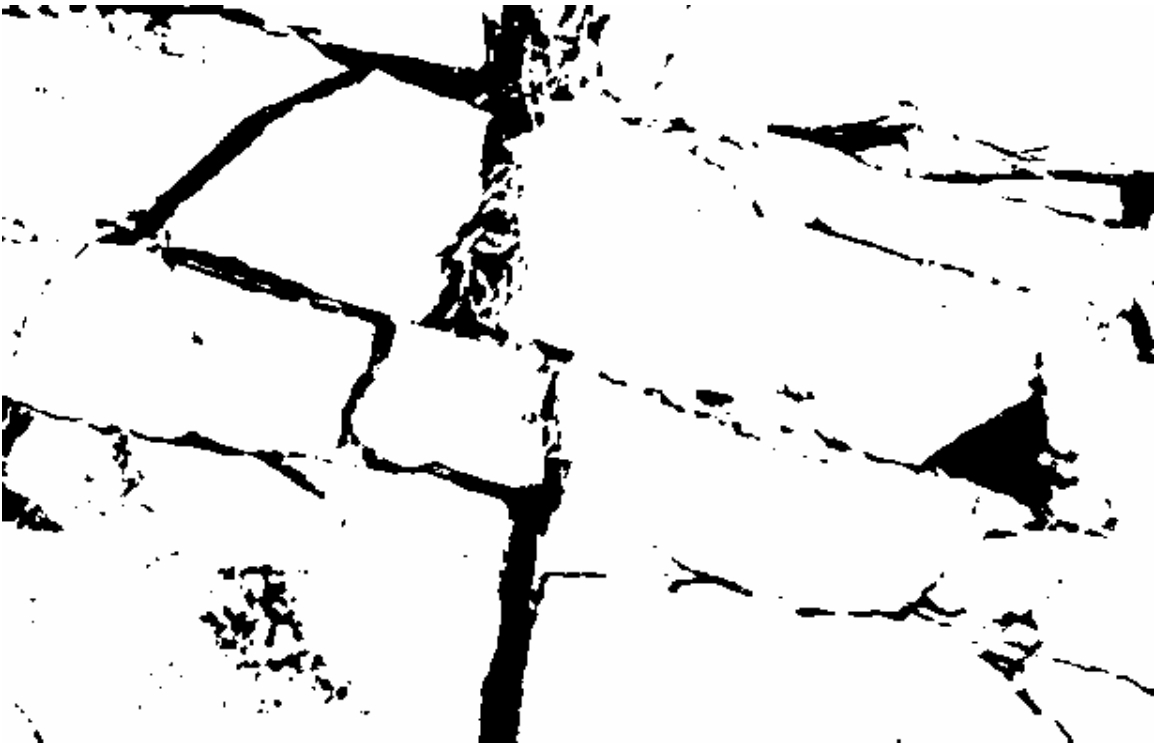
Figure 5.39. Smoothed binary image at threshold value of 100.
