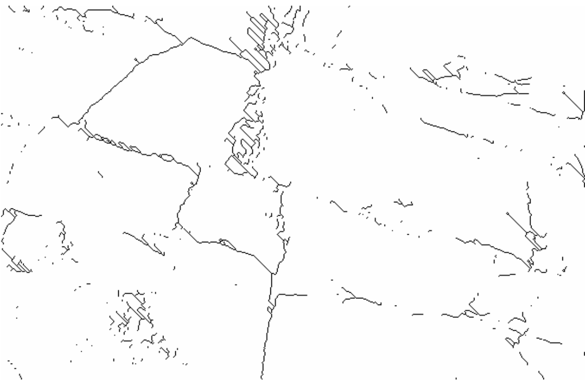
Figure 5.22. Thinned image using Hilditch's algorithm after single pass 3X3 smoothing and threshold of 100.
