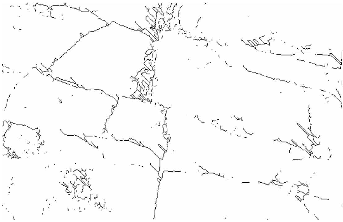
Figure 5.29. Thinned image using Hilditch's algorithm after threshold of 100 without smoothing.
