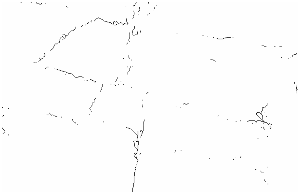
Figure 5.23. Thinned image using Hilditch's algorithm after single pass 3X3 smoothing and threshold of 50.
