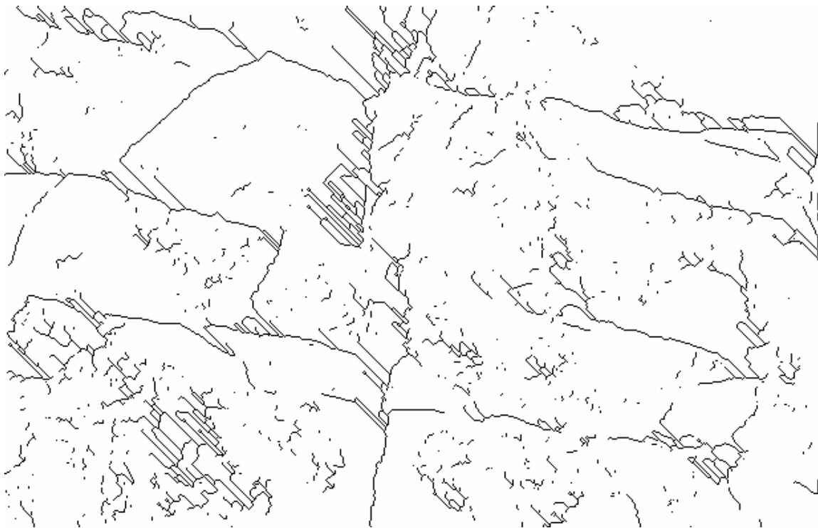
Figure 5.21. Thinned image using Hilditch's algorithm after single pass 3X3 smoothing and threshold of 128.
