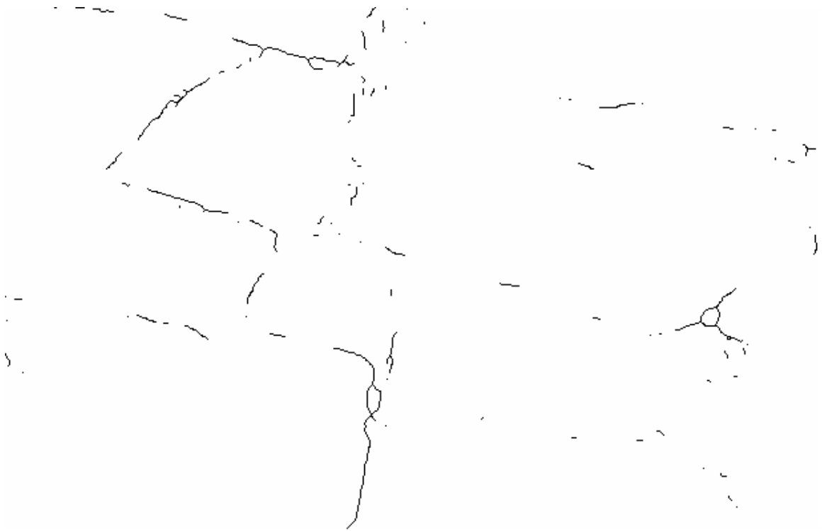
Figure 5.27. Thinned image using Zhang & Suen algorithm after single pass 3X3 smoothing and threshold of 50.
