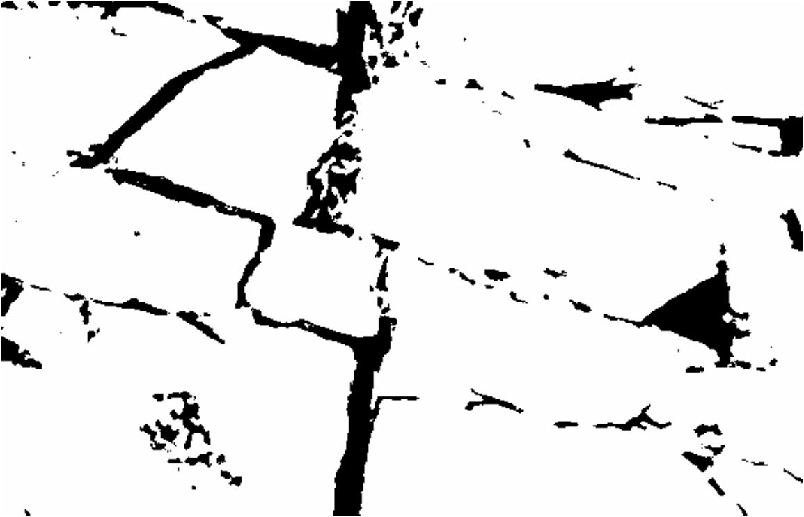
Figure 5.15 Binary image with threshold value of 100 after five pass 3X3 median smoothing.
