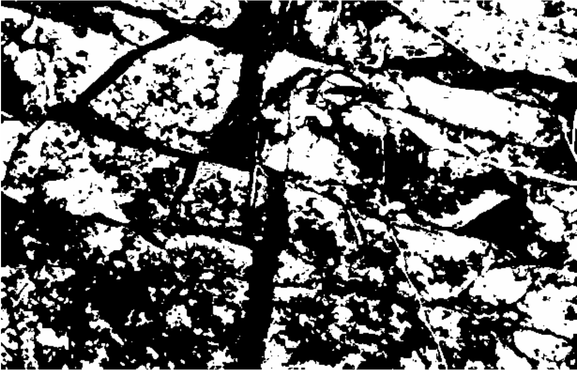
Figure 5.9. Binary image with threshold value of 150 after single pass 3X3 median smoothing.
