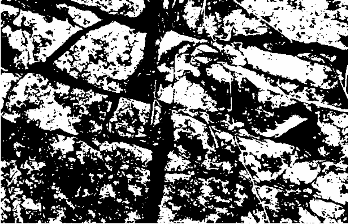
Figure 5.16. Binary image with threshold value of 150 without smoothing.
