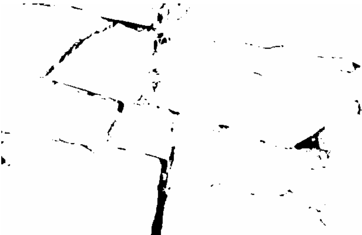
Figure 5.13 Binary image with threshold value of 50 after single pass of a 3X3 median smoothing.
