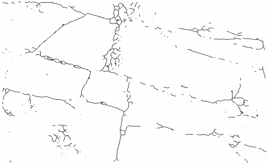
Figure 5.26. Thinned image using Zhang & Suen algorithm after single pass 3X3 smoothing and threshold of 100.
