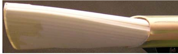
Figure 2-9. Linear twist distribution due to internal actuation. The compliant wing profile was manually cut from a closed-cell polyethylene wing. In addition to a rough exterior surface, the structure was incapable of supporting adequate wing loading.
