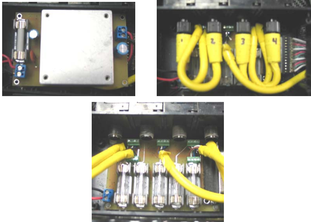
Figure 3-24. EPC Unit One. The top board is a DC/DC converter to clean the source power. Picture B shows the output ports from the valve board connected to the proportional flow valves. Picture C displays the actual valve board which protects and routes data to the valves.
