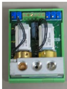
Figure 2-5. Electro-pneumatic pressure regulator. Internal solenoids track a high frequency PWM signal to track a command pressure value.
