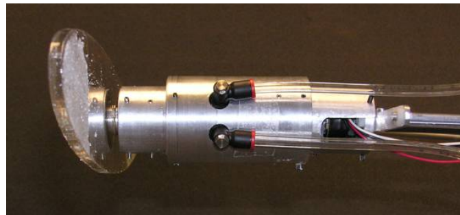
Figure 2-8. Internal and external view of twist mechanism. Significant torque output is produced by the series combination of the pneumatic rotary actuator and the planetary gear set. The gear friction helps the actuator to maintain static positioning.
