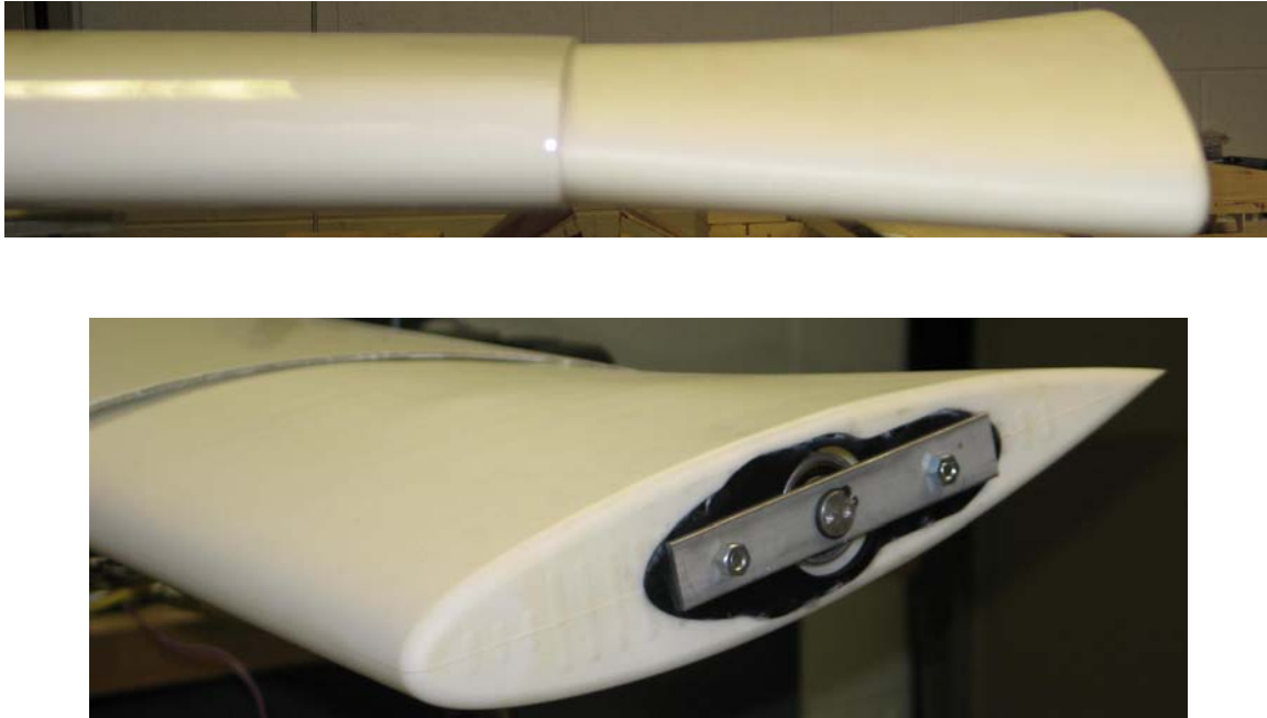
Figure 3-23. Twisting the Compliant Wings. A smooth contour is achieved by combining the internal twist mechanism and the compliant external structure.
