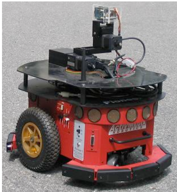
Figure 2.2: MobileRobots Pioneer 3-DX Ground Vehicle with Digital Camera Mounted on a PTU.
