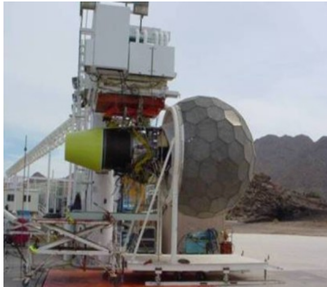
Figure 11. Photograph of the TECH977 engine mounted in the test stand. An inlet flow control device can be seen mounted around the engine inlet [30].
