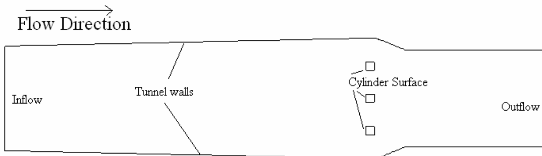
Figure 4.2 Computation grid for the three-cylinder configuration.
