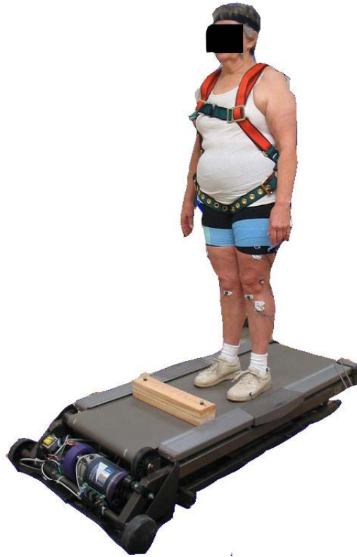
Figure 1: Trip recovery training experimental setup. Participant stood on an inactivated treadmill with an obstacle in front of their feet. Upon activation, the perturbation displaced the feet posteriorly so that the body center-of-mass was anterior to the base of support (similar to what one would experience in an actual trip).
