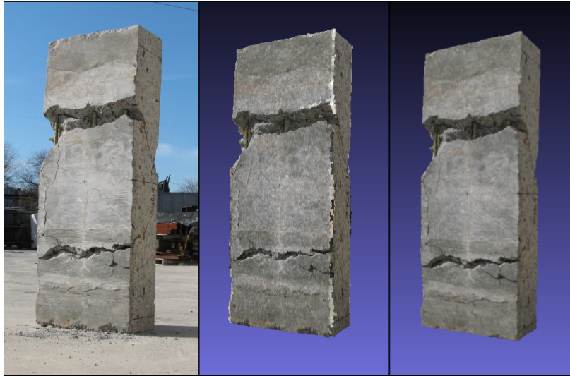
Figure 5.8: From left to right, a photo of the concrete column, the point cloud model, and the Poisson mesh model.
