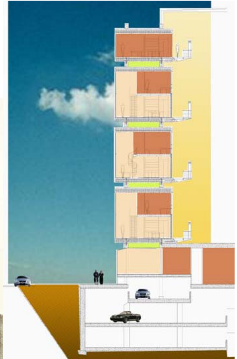
Partial Building Section showing parking, retail, residential, open space and utility chases.
