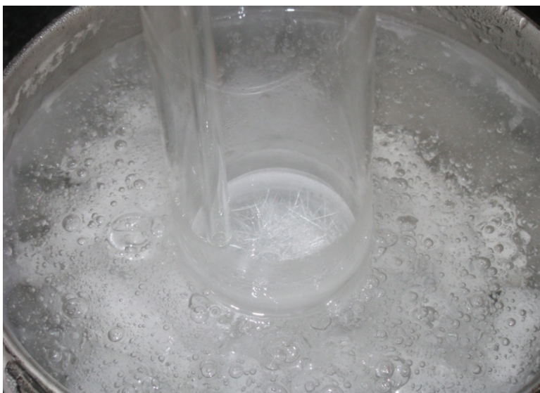
Figure 4.7 – N 2 O 5 crystals collecting at the base of the trapping vessel.
