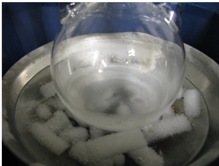
Figure 4.3 – White powder, supposedly N_2O_5 , collected in the round bottom flask after one hour of trapping.
