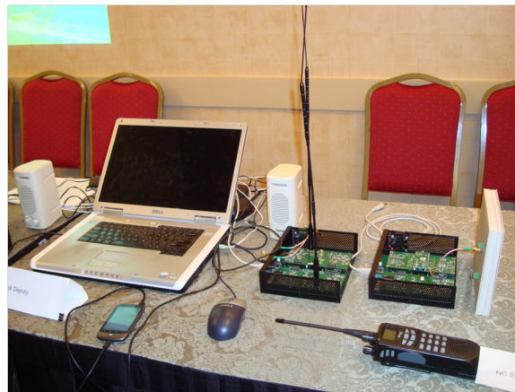
Figure 5.12: The PSCR Gateway Function as Implemented on a Laptop Computer
