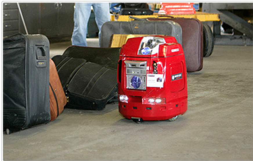
Figure 1.1: A wheeled security robot that is restricted to flat surfaces and ramps [2].
