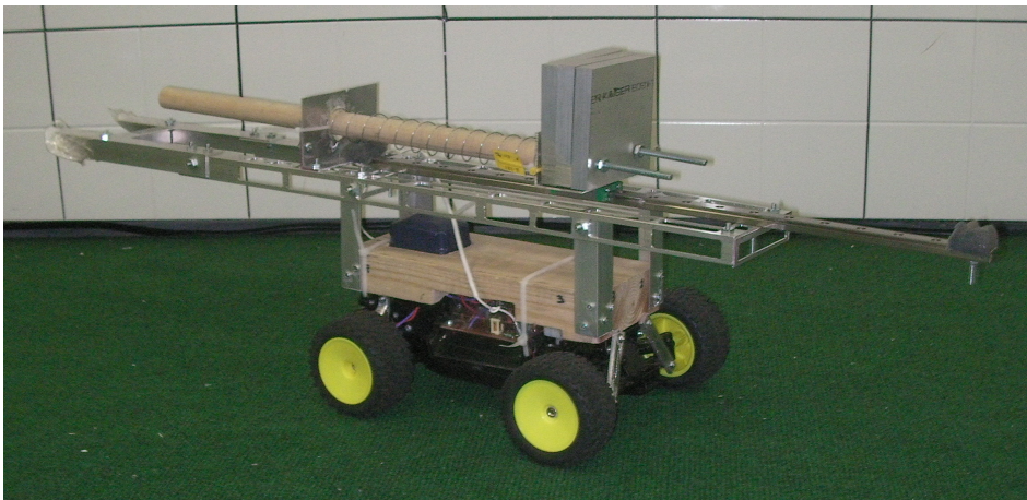
Figure 4.7: A robot designed using simulations to reduce the height of the slider for step-climbing.
