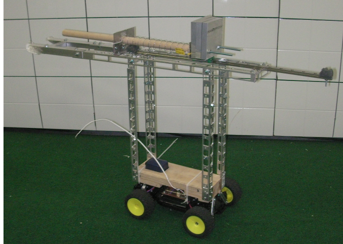
Figure 4.3: A robot equipped with a passive dynamic system to enable step-climbing. This robot was used to validate simulations and was designed to be excessively tall.
