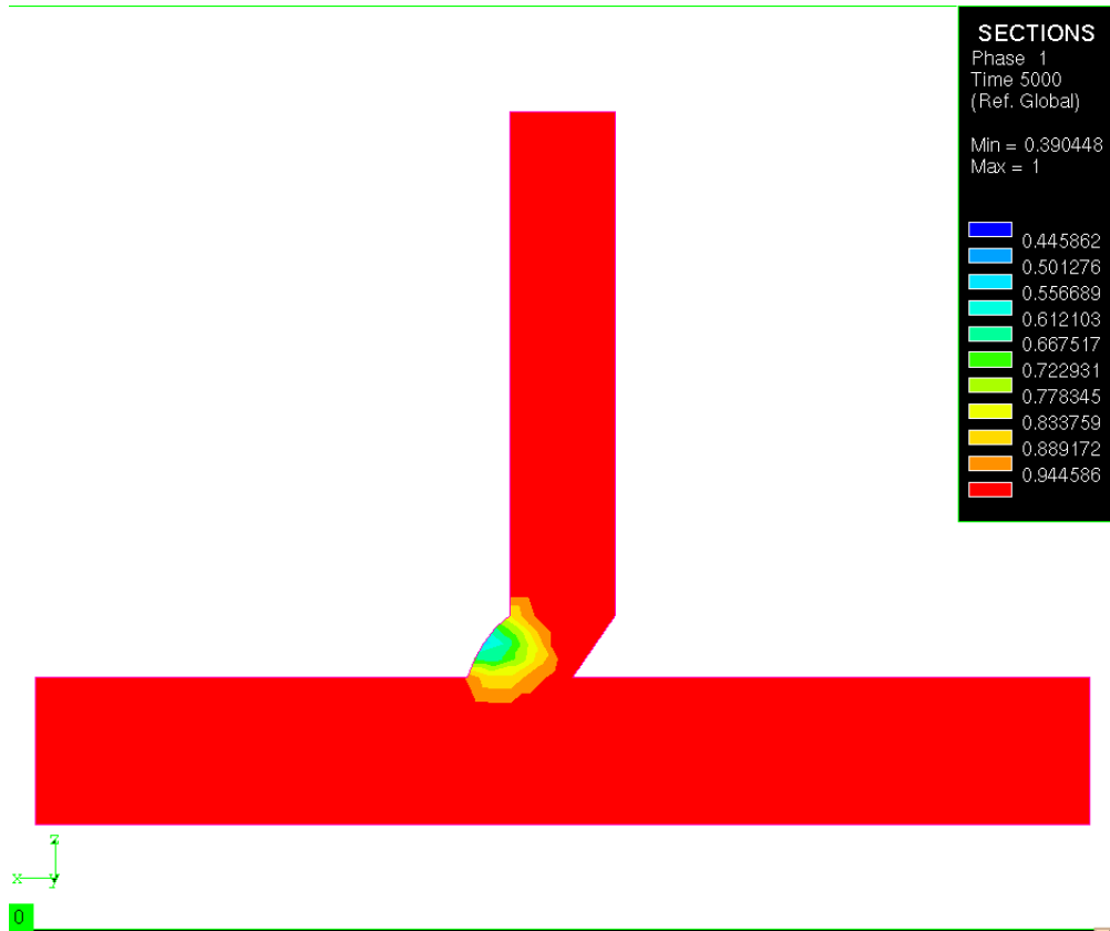
Fig. 6.25 Distribution of phase 1 material over the cross section after the first weld pass of the tee joint at t = 5000s
