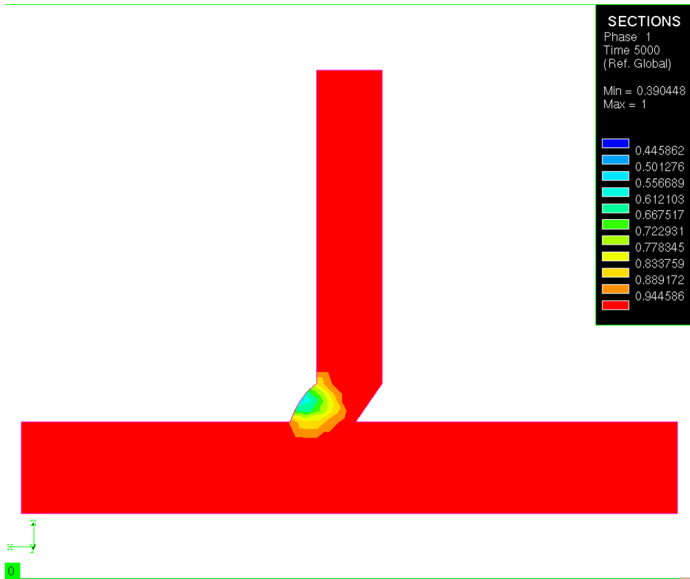
Fig. 7.5 Distribution of the phase 1 material over the cross section after the first weld pass of the tee joint at t = 5000s
