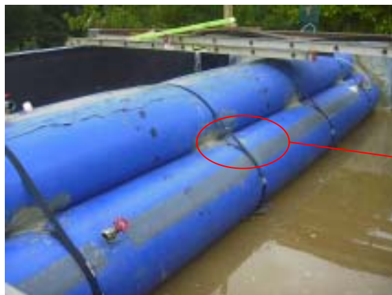
Figure 2-22: Bentonite Paste Applied to Strap Locations on Tube #2 and Tube #3 in Trial 4
