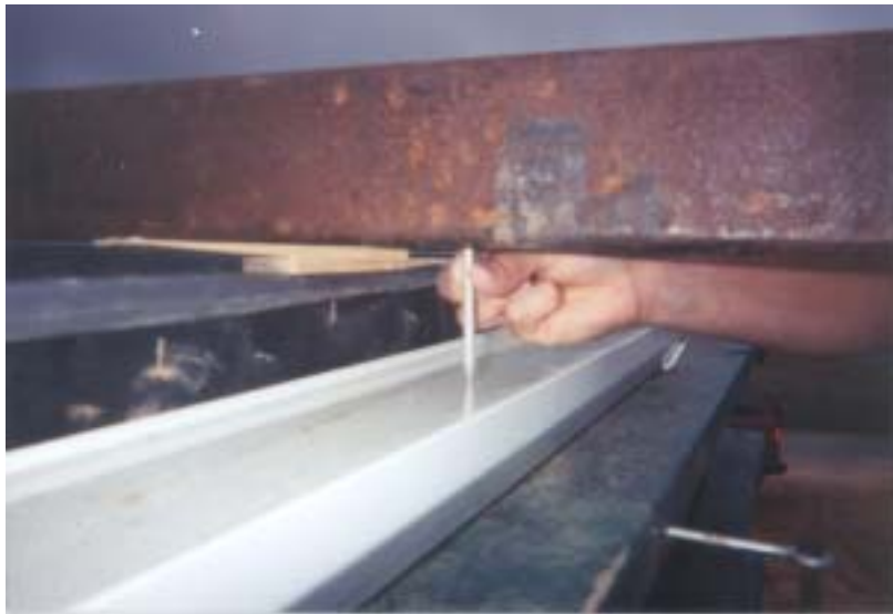
Figure 2-6: Aligning of the Measurement Beam in Vertical Direction
