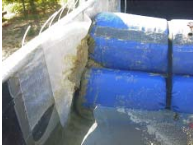
Figure 2-39: Trial 12 Just After Sliding Failure
