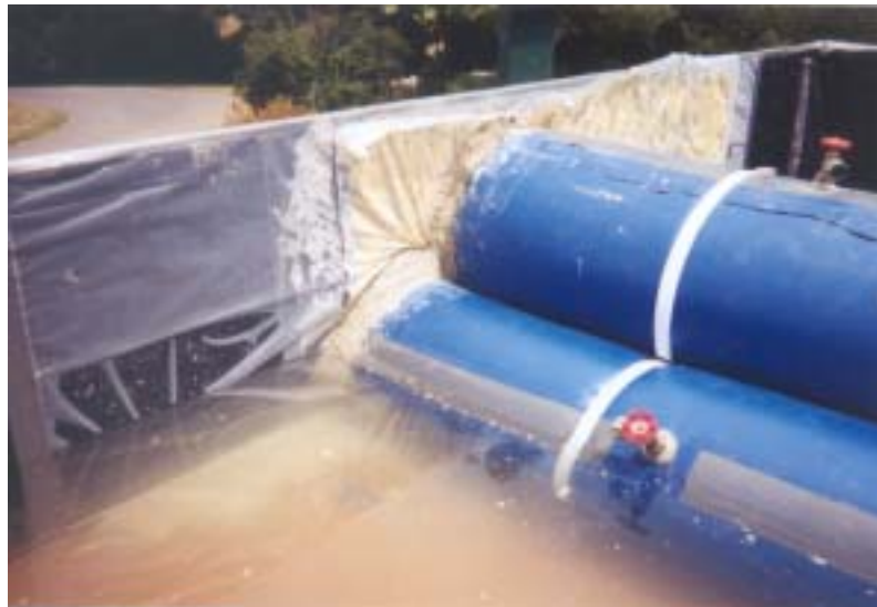
Figure 2-13: Tube #2 Rolling Away from Headwater at 7.5-Inch Water Height in Trial 1
