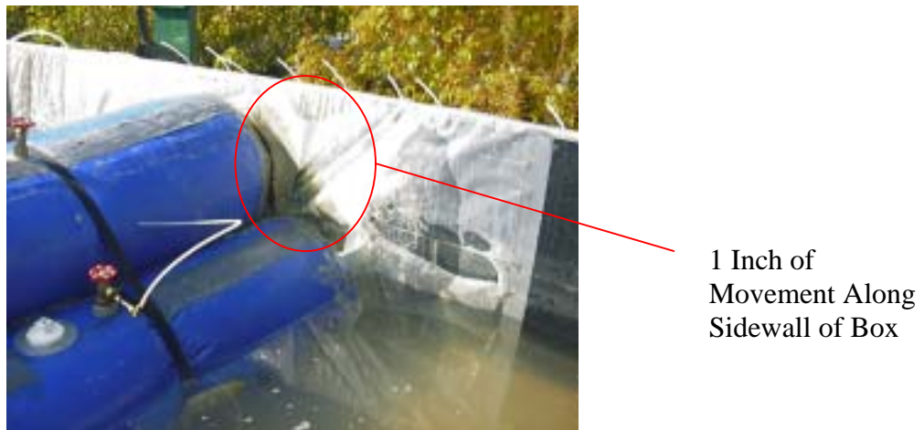
Figure 2-37: Trial 11 Just After Sliding Failure
