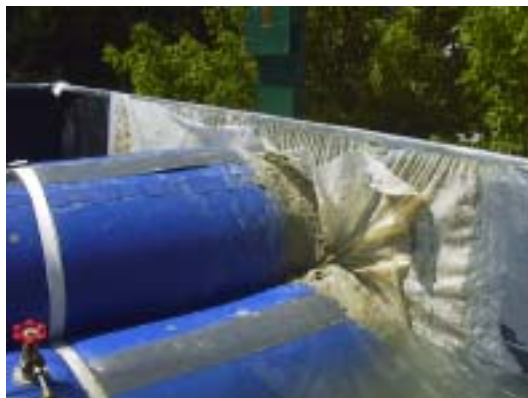
Figure 2-15: Rotation of Tube #2 Against Sidewall of Box at 10-Inch Water Height in Trial 2
