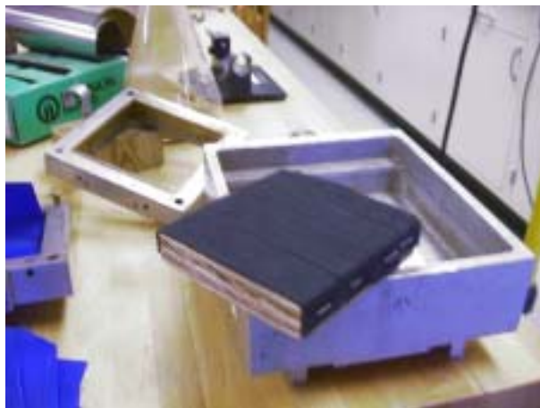
Figure 2-43: Strapping Material Attached to the Wooden Block
