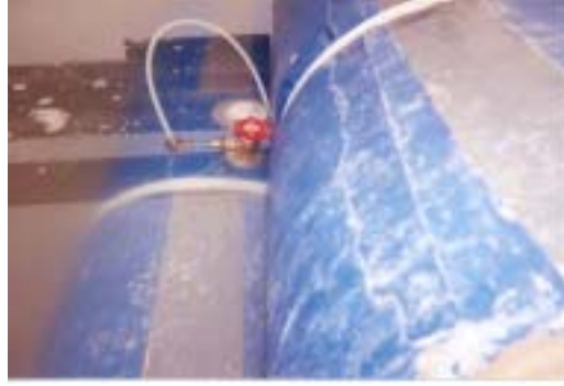
Figure 2-18: Valve on Tube #2 Nearly Sheared Off by Tube #3 in Trial 3
