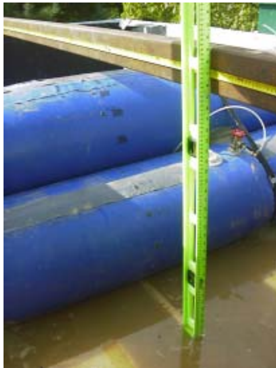
Figure 2-7: Measurement Tool for Obtaining Measurements Under the Tubes
