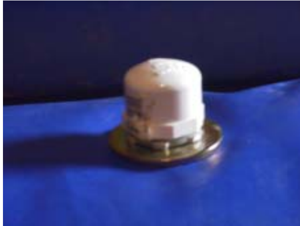
Figure 2-2: Release Drain Installed on Existing Tube
