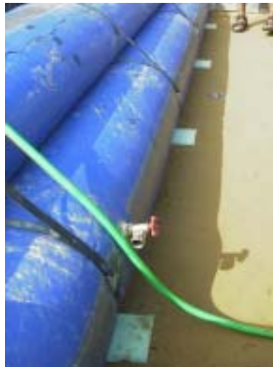
Figure 2-30: Foam Material Placed under Strap Locations for Trial 7
