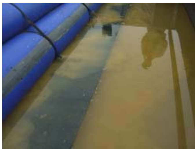
Figure 2-33: Beginning of Piping Failure on Tailwater Side of Tubes in Trial 9
