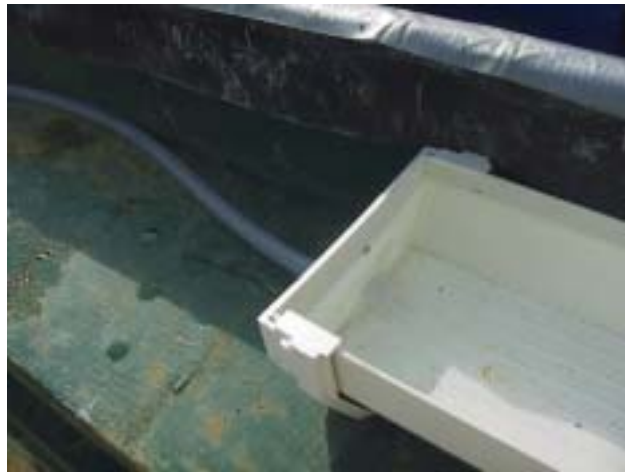
Figure 2-3: End Cap and Connecting Hose Used in Leveling Trough
